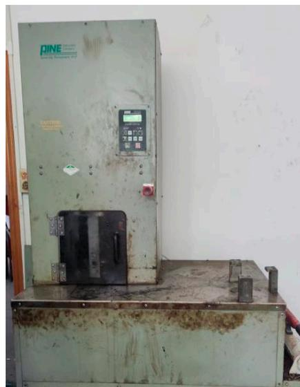
Figure 2. Superpave gyratory compactor.
