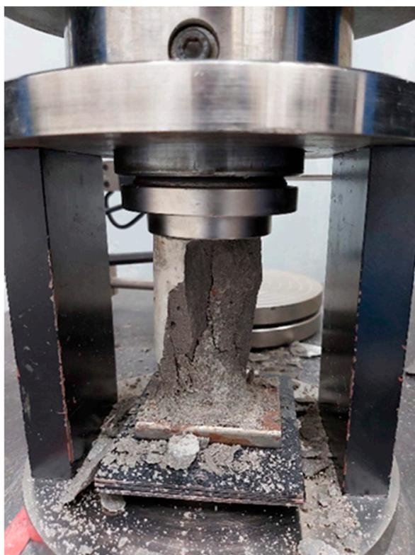
**Figure 7.** Cylindrical mortar samples after the compression test.
