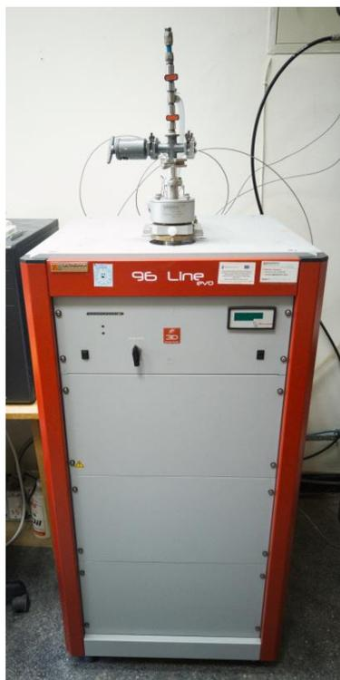
**Figure 1.** Setaram MHTC 96 Line evo calorimeter.
