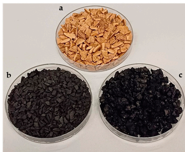
Figure 1. Starting walnut shells (a) and activated biocarbons obtained by direct (b) and chemical activation (c).
