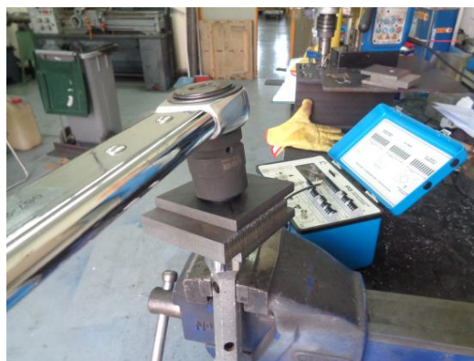
Figure 6. Strain gauge calibration with torque wrench.
