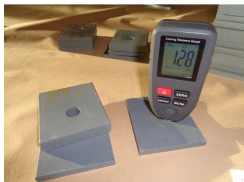
Figure 4. Coating thickness measurement.
