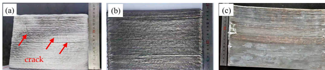
Figure 1. Thin-walled alloy components prepared by WAAM: (a) Al-Mg-Si, (b) TB, (c) TC.
