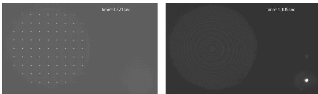
At this point we want to remark one of the characteristic of VPTNLCs, flexibility. We can use the same VPTNLC cell for measuring and compensating the wavefront aberration. Additionally we can align by software the sampling array and the compensation element with the exit pupil of the optical system easily by displacing the projection coordinates of the images, alignment with a precision of one pixel.
