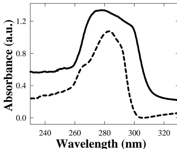
In Figure 6, the absorption spectrum of our polycarbonate films with dispersed TGNPs is reported. As comparisons with Figures 3 and 5 suggest, the low wavelength range spectrum is mostly dominated by the polycarbonate absorption; the fingerprint of the TGNPs is present above 450 nm, approximately. At growing nanoparticle concentration with respect to PC from 1‰ up to 6‰ we observe the increase of TGNP absorption band centered around 545 nm, irrespective of TGNP concentration.
