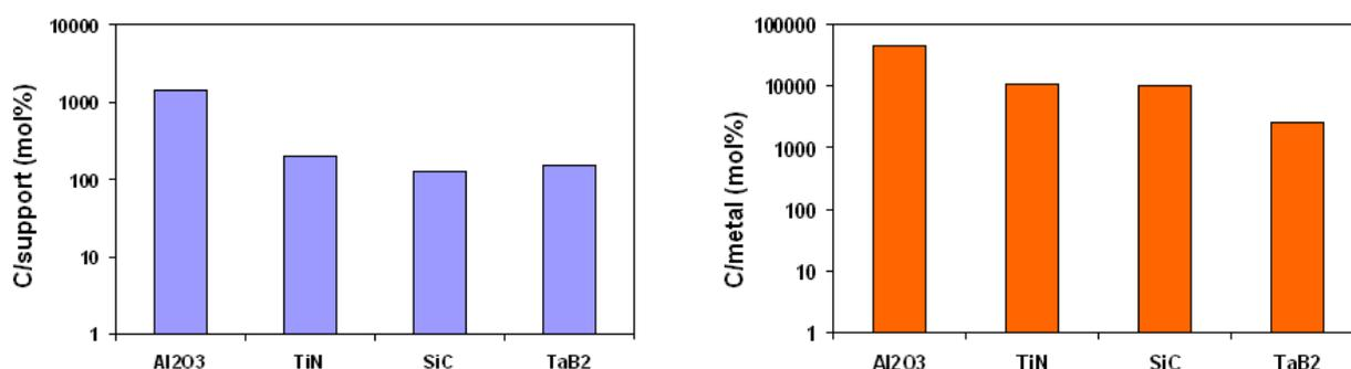
As can be seen in Figure 8, the reaction path also affects the yield of carbon nanotubes produced. At temperatures below 500 °C, the oxidative dehydrogenation reaction follows the reaction (1). When the
