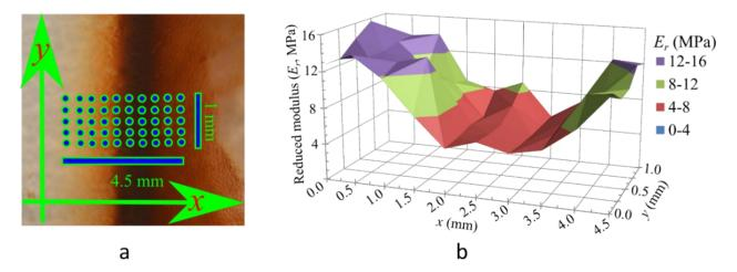
Figure 3. Heterogeneity in  $E_r$ . (a) Sample with  $\psi^* = 0.1\%$  shows that MNP concentration is highest in the region immediately above the periphery of the magnet. Approximate locations of indentations are shown with dots; (b) Map of  $E_r$  obtained from indentation at such points on a sample with  $\psi^* = 1.0\%$  shows that variations in  $E_r$  roughly match variations in  $\psi$ .
