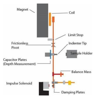
**Figure 5.** Schematic of the NanoTest<sup>®</sup> instrument. The indenter is attached to a pendulum that can rotate around a virtually frictionless pivot. The indenter is loaded against the sample by passing a current through the coil, which is then drawn to the permanent magnet. Displacement of the indenter into the sample is measured by the variation in voltage between the capacitor plates.
