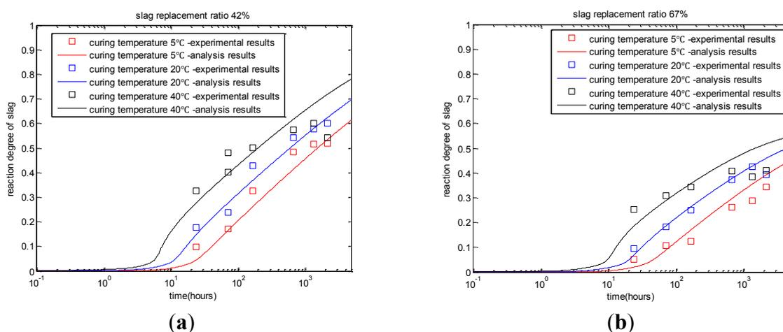
**Figure 1.** Reaction degree of slag with different slag replacement ratios and curing temperatures (experimental results are taken from reference [15]). (a) cement-slag paste with 42% slag; (b) cement-slag paste with 67% slag.
