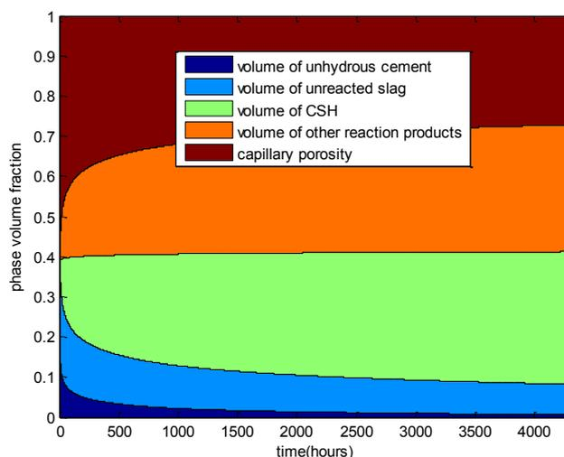
**Figure 7.** Phase volume fraction evolutions of cement-slag paste: water-to-binder ratio of 0.5, slag replacement ratio of 0.5.
