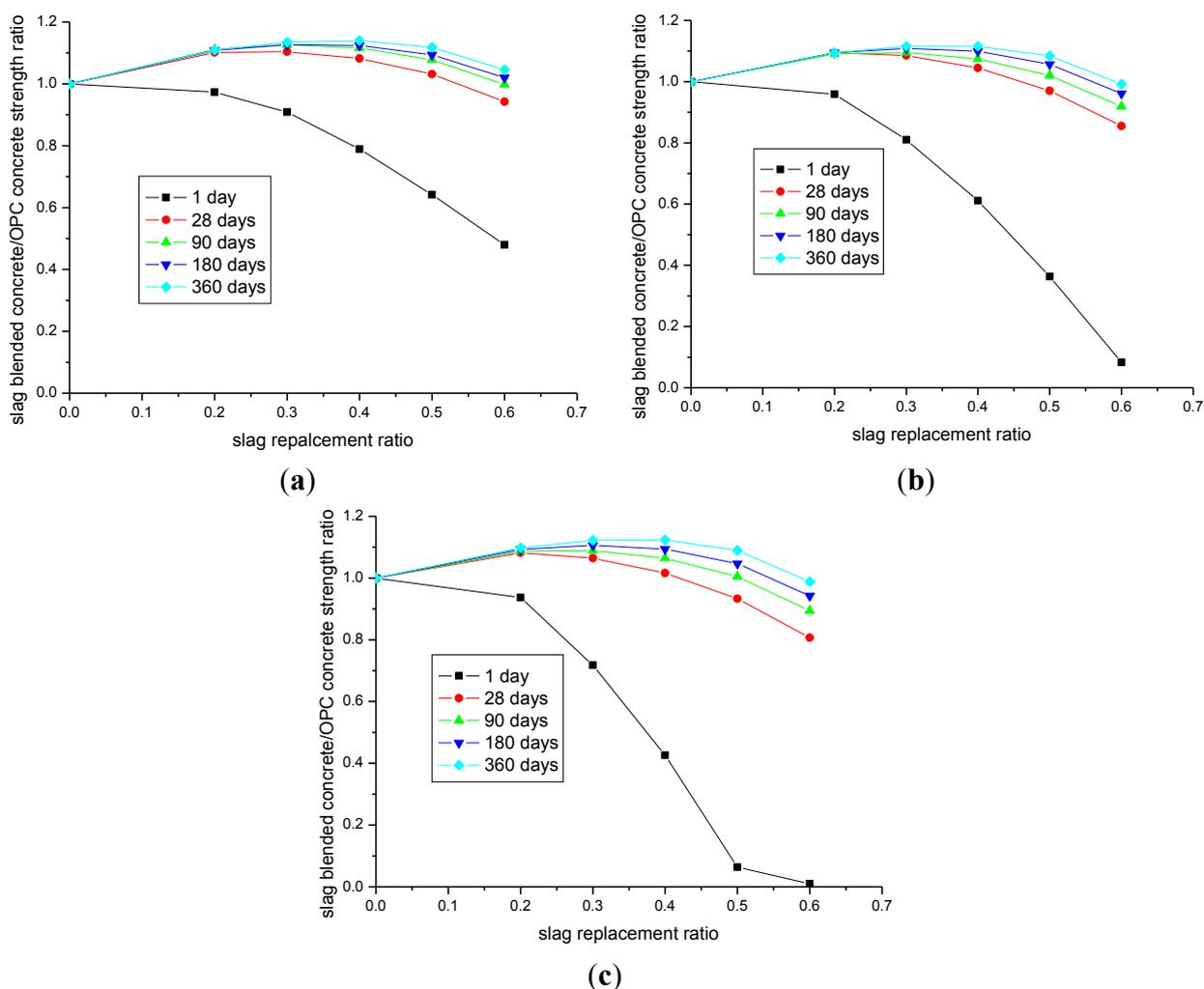
**Figure 8.** Effects of slag inclusions on the compressive strength development of concrete. (a) water-to-binder ratio of 0.35; (b) water-to-binder ratio of 0.5; (c) water-to-binder ratio of 0.7.
