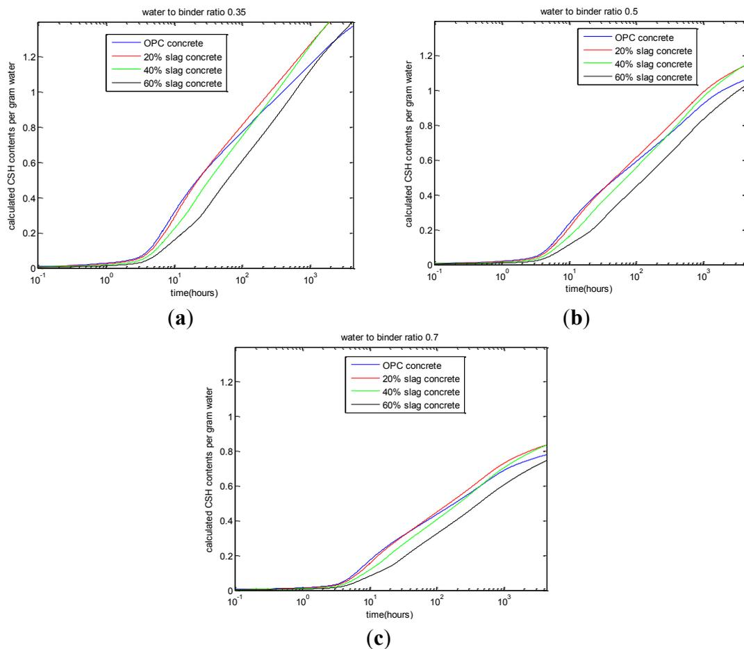
Figure 4. Calculated calcium silicate hydrate (CSH) content. (a) water-to-binder ratio of 0.35; (b) water-to-binder ratio of 0.5; (c) water-to-binder ratio of 0.7.
