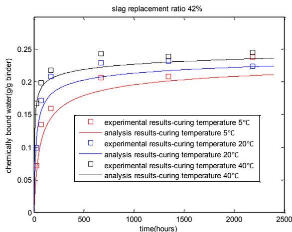
**Figure 2.** Evaluation of chemically bound water of cement-slag blends (water-to-binder ratio of 0.42) (experimental results are taken from reference [15]).
