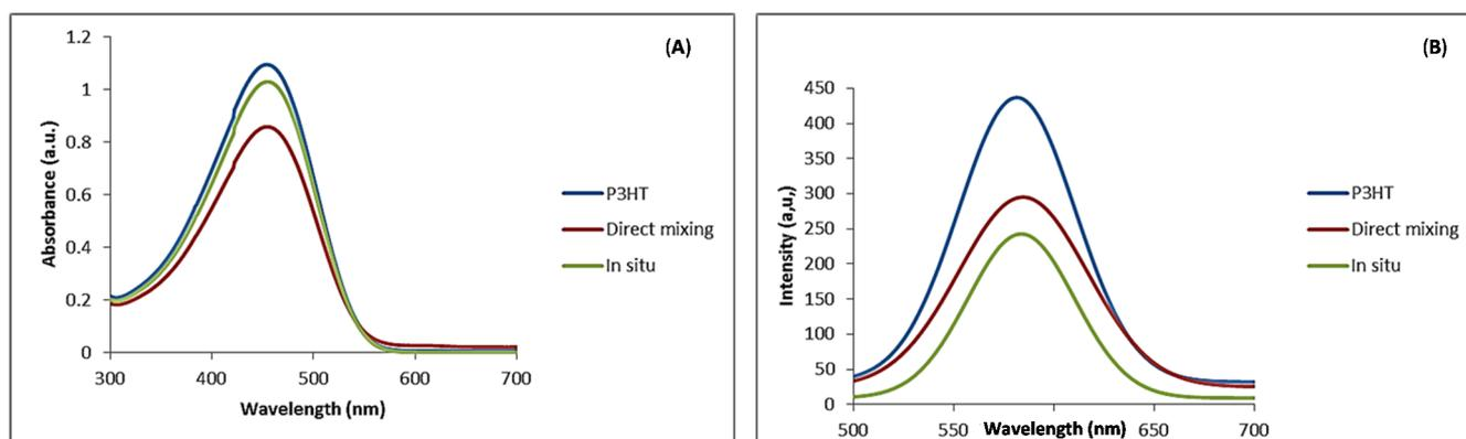
**Figure 6.** (A) Uv-Vis absorption spectra; (B) photoluminescence emission for P3HT and P3HT/N-CNTs nanocomposites in chloroform solution.
