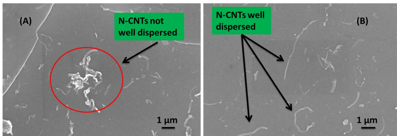
**Figure 10.** SEM images of the cell morphology showing N-CNTs (A) not well dispersed in the direct mixing nanocomposite; and (B) well dispersed for the *in situ* polymerization nanocomposite.
