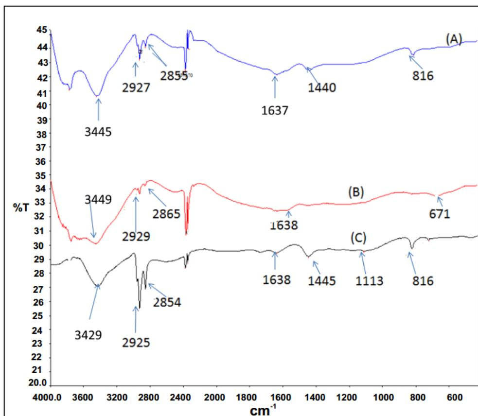
**Figure 5.** FTIR absorption frequencies for P3HT and nanocomposites (A) P3HT; (B) *in situ*; (C) direct mixing.
