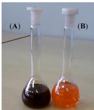
**Figure 3.** Color of P3HT in chloroform solution (A) after formation of nanocomposite and (B) pristine P3HT under white light.
