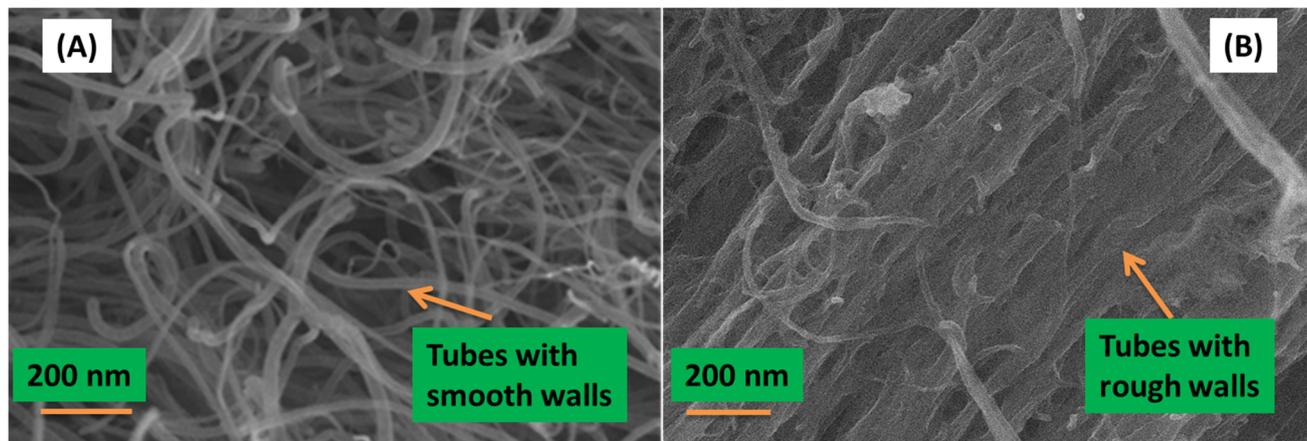
**Figure 2.** Morphology of (A) N-CNTs; and (B) nanocomposite of N-CNTs/P3HT synthesized by *in situ* polymerization.
