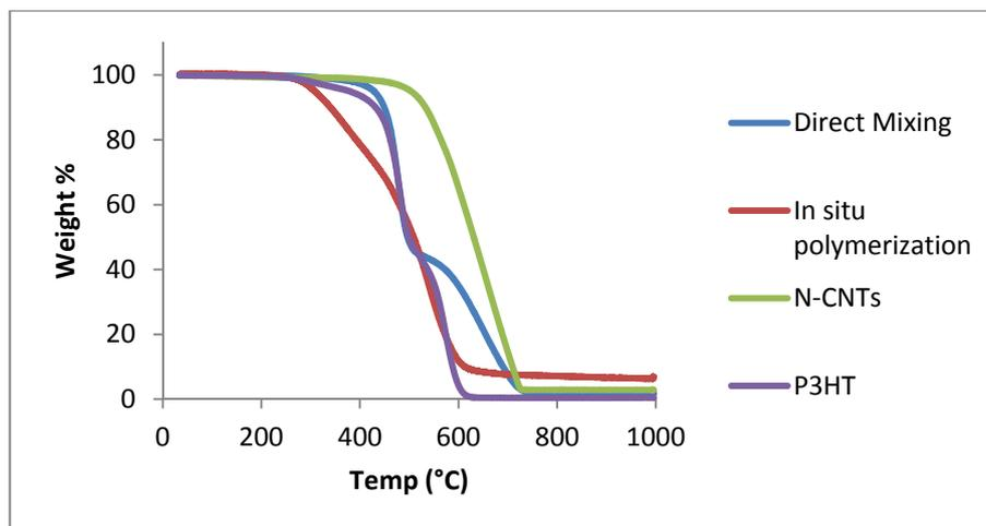
**Figure 7.** Thermogravimetric analysis of N-CNTs, P3HT and P3HT/N-CNTs nanocomposites.
