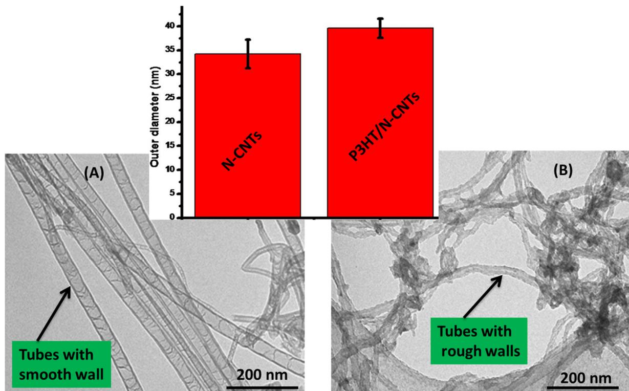
**Figure 1.** TEM images of (A) purified N-CNTs; and (B) N-CNT/P3HT nanocomposite synthesized by *in situ* polymerization (inset comparison of outer diameters).
