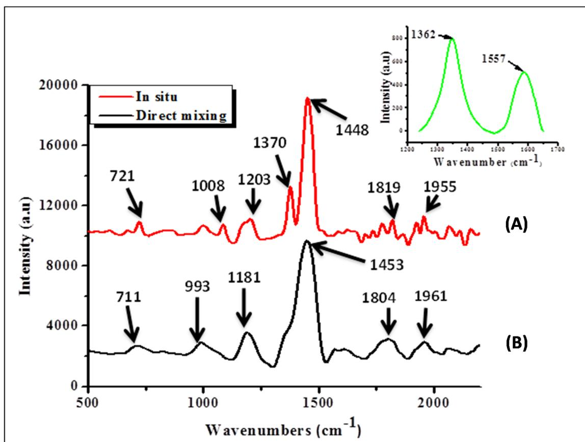
**Figure 4.** Raman spectroscopy results of nanocomposites, (A) direct mixing and (B) *in situ* polymerization (inset position of D-band and G-band for N-CNTs).
