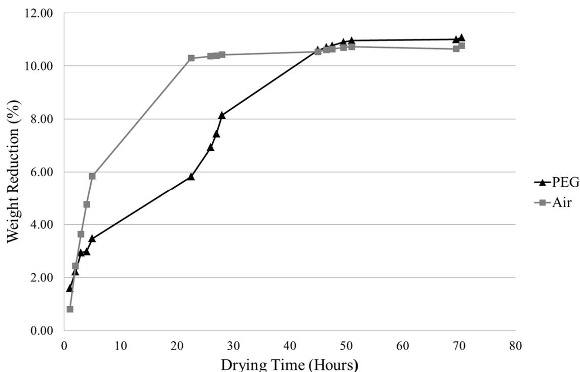
**Figure 1.** Comparison of sample weight reduction by PEG drying and air drying at 62% solid loading and using desiccant PEG4000 in a 30% concentrated aqueous solution.
