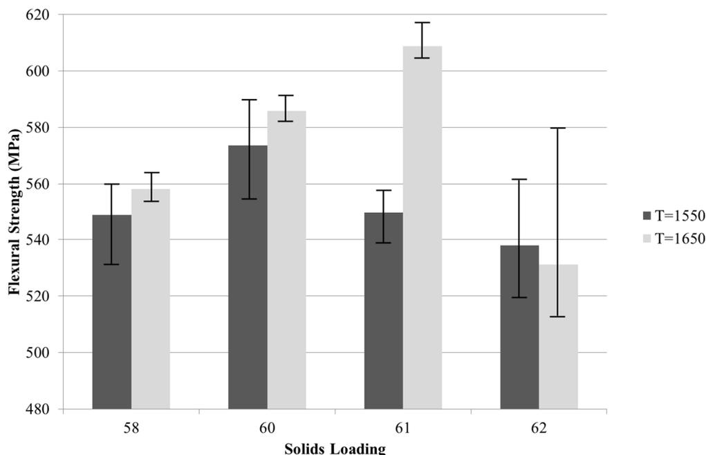
**Figure 9.** Flexural strength obtained from three-point bend testing for solid loadings ranging from 58%–62% at sintering temperatures of 1550 °C and 1650 °C.
