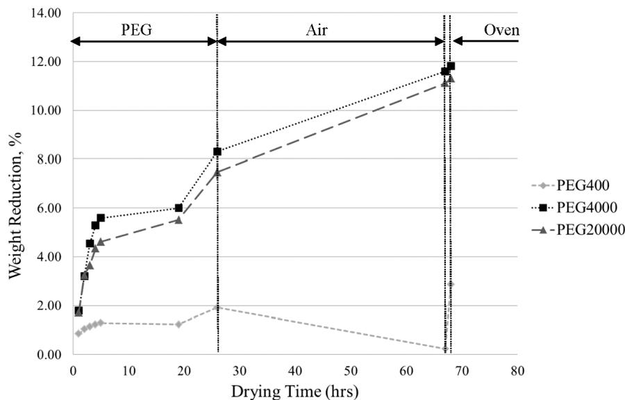
**Figure 2.** Sample weight reduction by PEG 400, 4000 and 20,000 at a 30% concentrated aqueous solution followed by air drying and oven drying.
