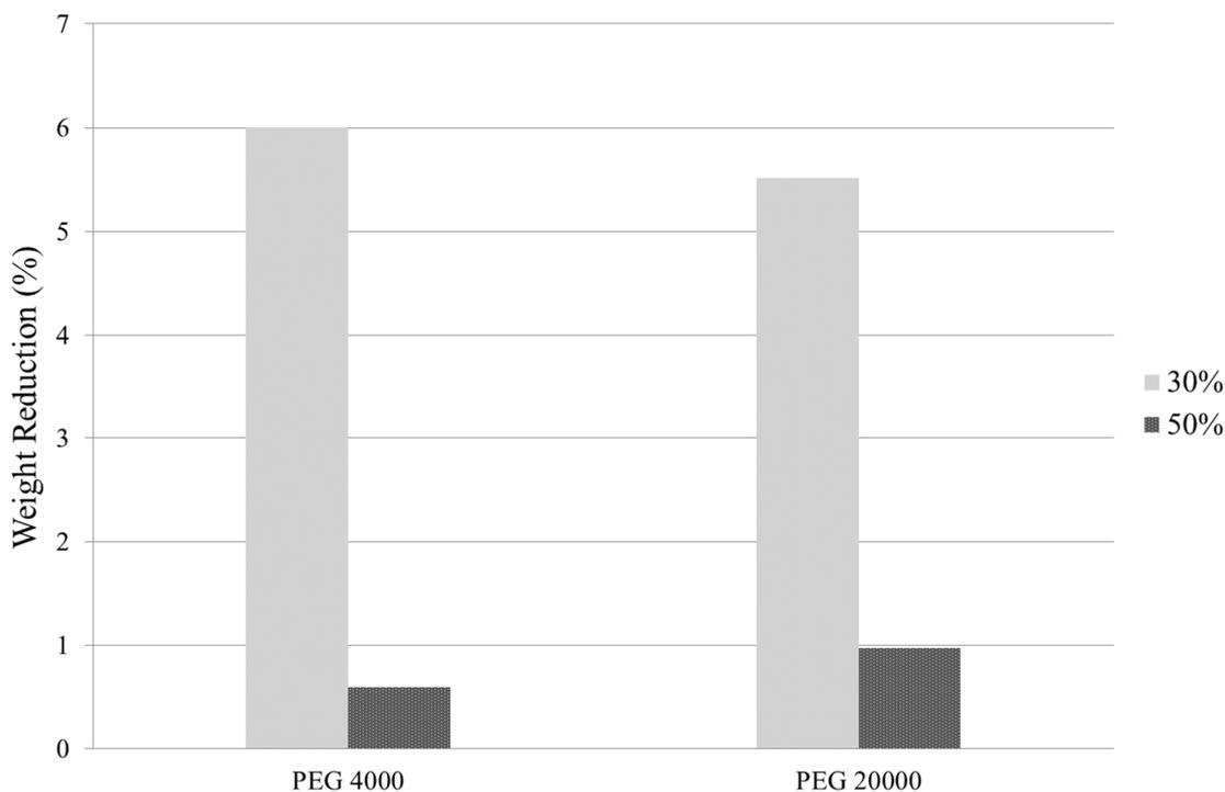
**Figure 4.** Sample weight reduction over the 20-h osmotic drying period using 30% and 50% conc. aqueous solution of PEG 4000 and PEG 20,000.
