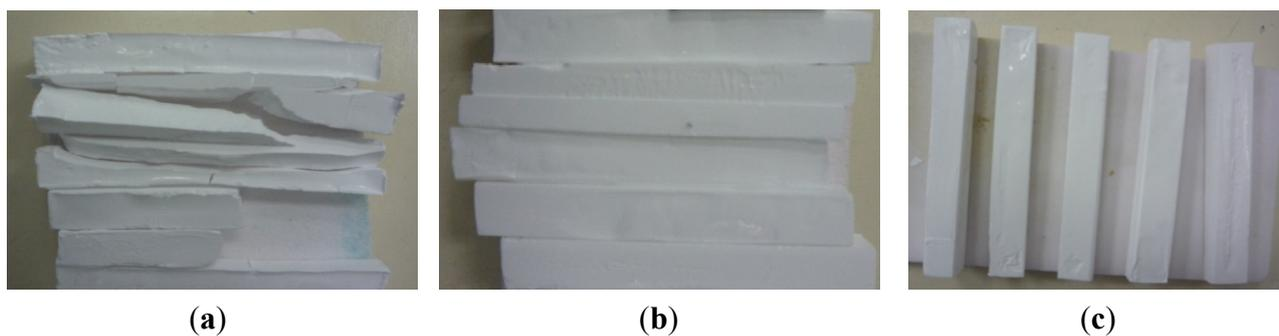
**Figure 3.** Sintered zirconia-toughened alumina (ZTA) parts after osmotic drying by: (a) PEG 400; (b) PEG 4000; and (c) PEG 20,000.
