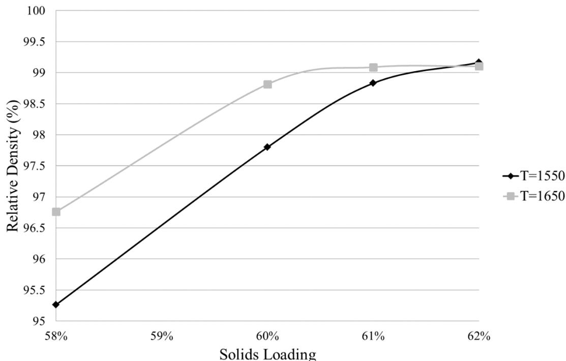
**Figure 5.** Relative density obtained at solid loadings ranging from 58%–62% at sintering temperatures of 1550 °C and 1650 °C.
