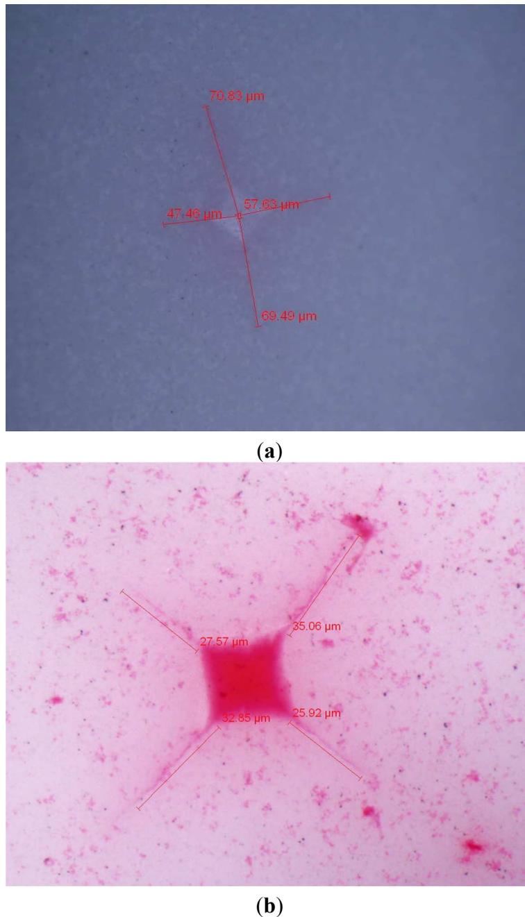
**Figure 8.** Optical micrograph of Vickers hardness indentation on ZTA surfaces conducted: (a) without colouring; (b) with red surface colouring.
