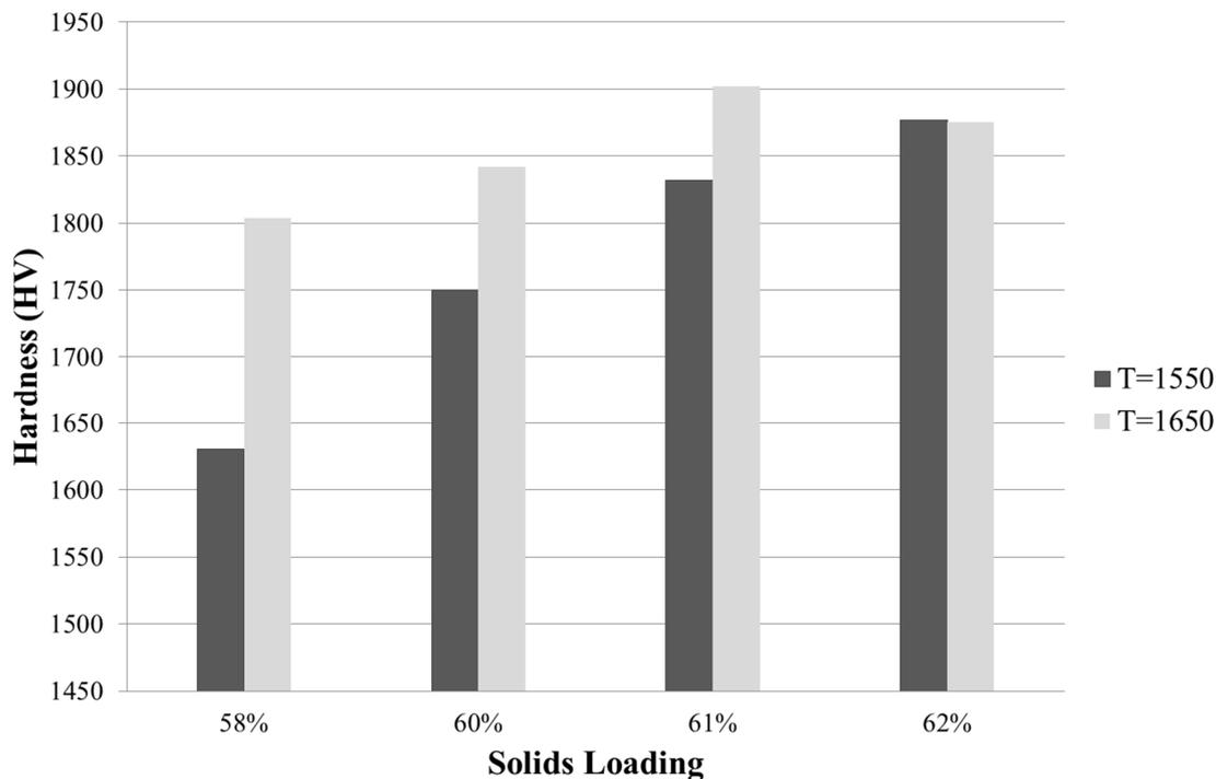
**Figure 6.** Vickers hardness obtained at solid loadings ranging from 58%–62% at sintering temperatures of 1550 °C and 1650 °C.
