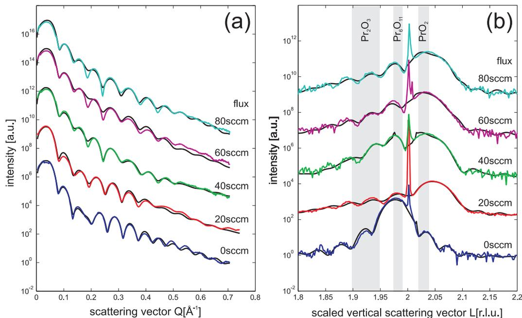
**Figure 4.** SR-XRR (a) and SR-XRD (b) data obtained from 9 nm praseodymia films using different  $O_2$  fluxes during plasma treatment (20–80 sccm) keeping other parameters (26 Pa  $O_2$ , 15 min treatment time) constant. The lowest flux of 20 sccm  $O_2$  is already sufficient to completely oxidize the praseodymia film.
