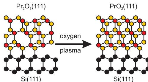
**Figure 5.** Schematic drawing of the plasma oxidation process. Randomly distributed oxygen vacancies in the  $\text{Pr}_2\text{O}_3$  film are occupied by oxygen from the oxygen plasma. The drawing considers also the B orientation of the praseodymia films with respect to the Si(111) support.
