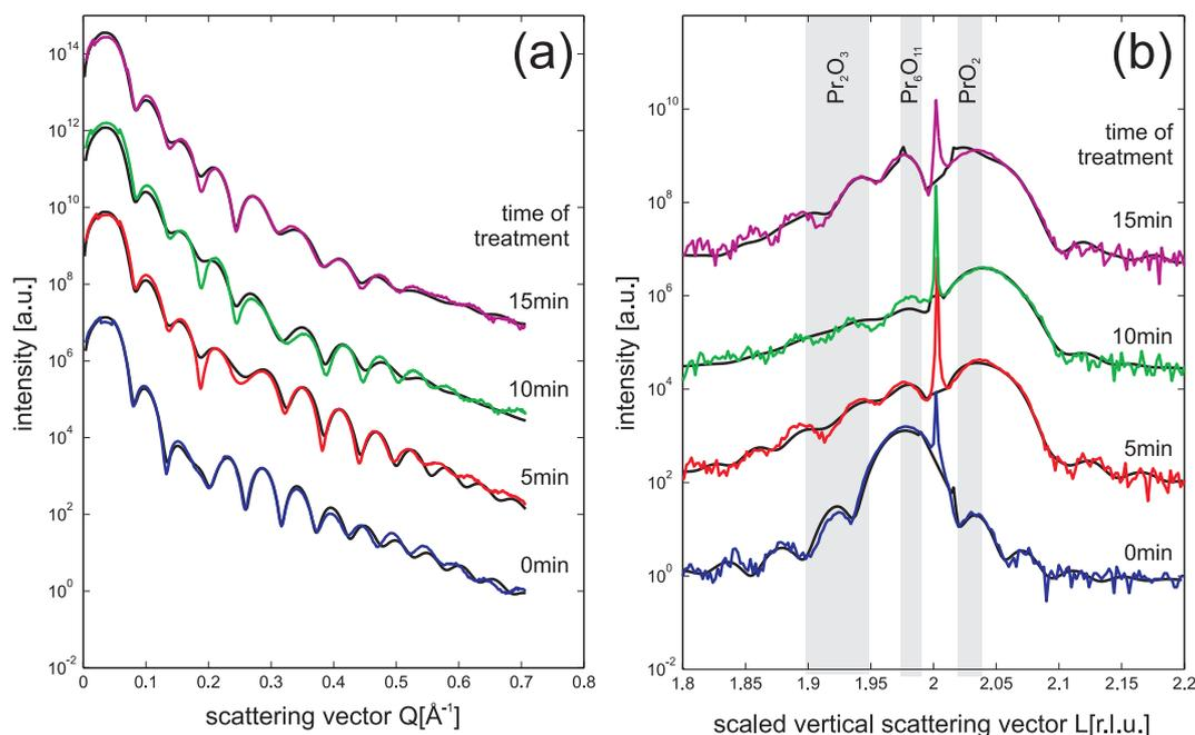
**Figure 3.** SR-XRR (a) and SR-XRD (b) data obtained from 9 nm praseodymia films after different plasma treatment times (5–15 min) keeping other parameters (26 Pa  $\text{O}_2$ , 40 sccm flux) constant. Complete oxidation is already obtained after the first 5 min oxidation step.
