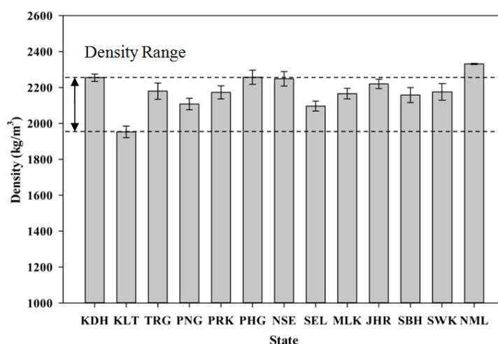
**Figure 12.** Variation in density for the samples of each state.
