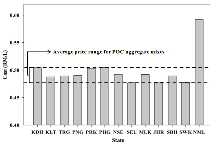
**Figure 18.** Cost of mortar incorporating POC aggregate (Kanadasan and Abdul Razak [32]).
