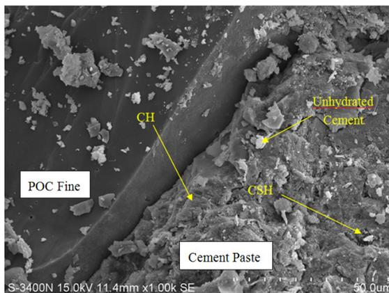
Figure 16. Aggregate cement paste interface.
