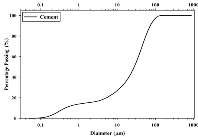
Figure 5. Particle size distribution for ordinary Portland cement (CEM I) 52.5N.
