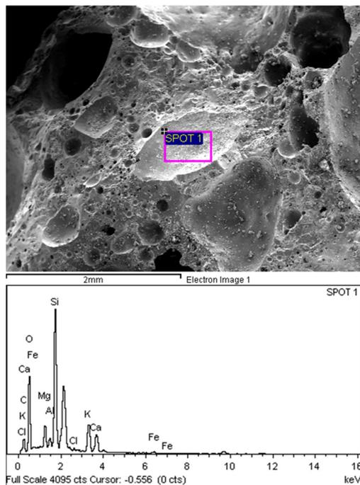
**Figure 8.** POC aggregate micrograph at a larger magnification.
