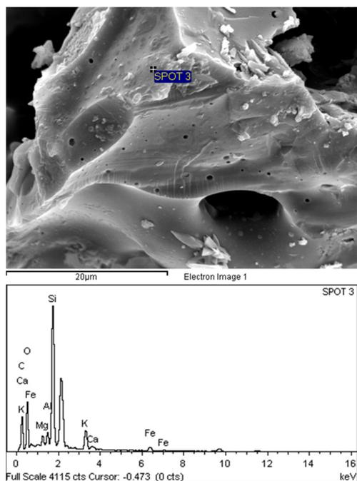
**Figure 9.** Presence of micro-pores within internal POC aggregate structure.
