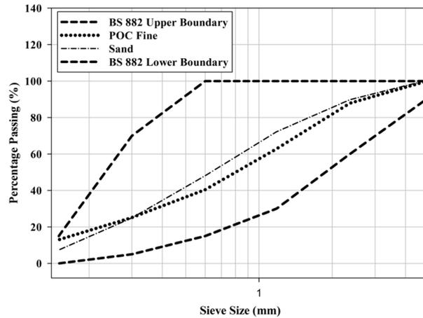
Figure 4. Particle size distribution for sand and POC fine.
