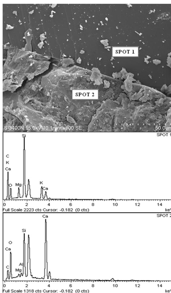
Figure 17. POC aggregate—Cement paste interface with X-ray spectroscopy (EDX).
