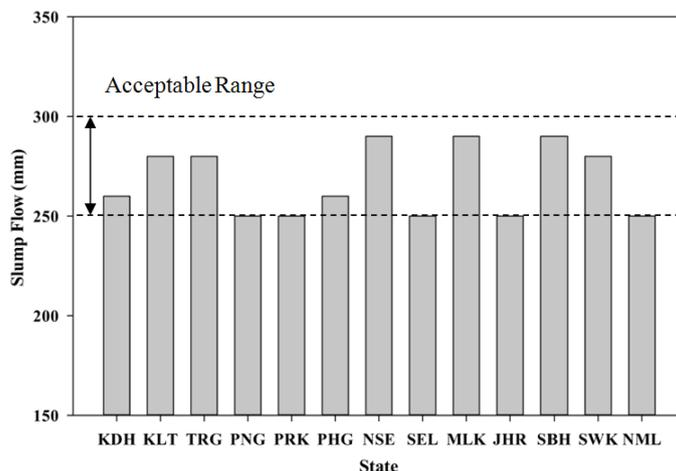
Figure 10. Slump flow test results.
