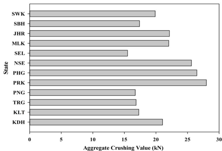
**Figure 6.** Aggregate crushing values for various states.
