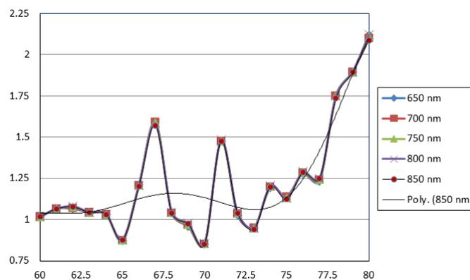
**Figure 4.** Dependence between the optical density and the temperature.
