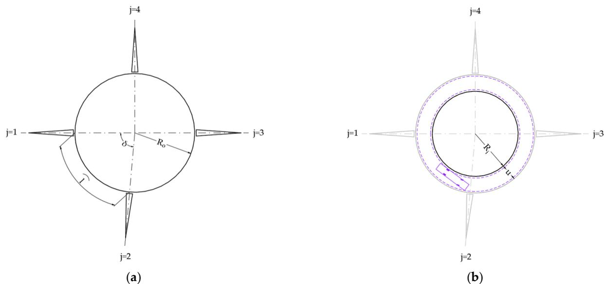
**Figure 1.** Design of initial geometric parameters: (a) the outer radius, legs, and splitter islands; (b) the central island radius and the circulatory roadway width defined based on the design vehicle swept path when driving in a full circle.
