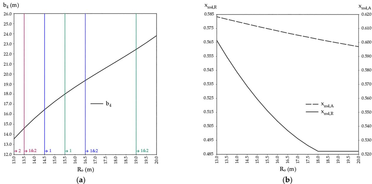
Figure 12. Investigated parameters at leg 4 as a function of  $R_o$  for different  $\delta$ , considering the application of design conditions 1 and 2: (a) geometric parameter  $b_4$ ; (b) traffic parameter  $x_{m4}$ .
