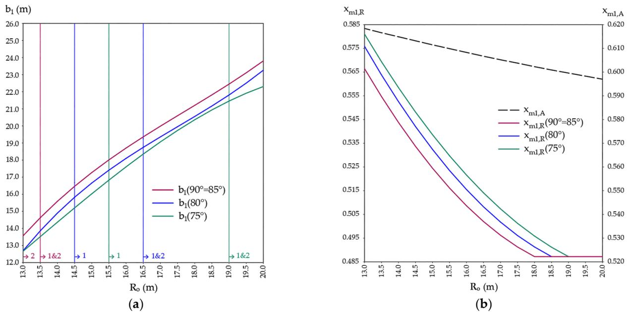
**Figure 9.** Investigated parameters at leg 1 as a function of  $R_0$  for different  $\delta$ , considering the application of design conditions 1 and 2: (a) geometric parameter  $b_1$ ; (b) traffic parameter  $x_{m1}$ .
