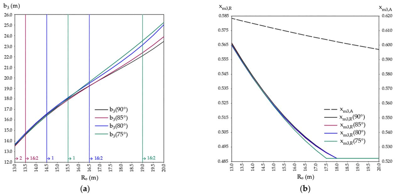
Figure 11. Investigated parameters at leg 3 as a function of  $R_o$  for different  $\delta$ , considering the application of design conditions 1 and 2: (a) geometric parameter  $b_3$ ; (b) traffic parameter  $x_{m3}$ .
