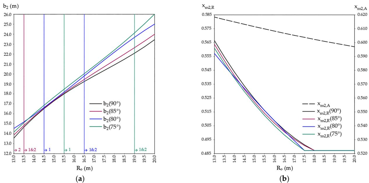
**Figure 10.** Investigated parameters at leg 2 as a function of  $R_0$  for different  $\delta$ , considering the application of design conditions 1 and 2: (a) geometric parameter  $b_2$ ; (b) traffic parameter  $x_{m2}$ .
