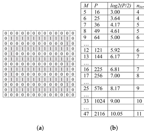
**Figure 11.** (a): a 13 × 13 image containing the longest perimeter zigzag object. (b): M = image width = image length. P = perimeter = ((M − 1) × (M − 2)) + 4 × ((M − 1)/4). log2(P/2) = theoretical number of iterations to compute jump distances for the 0-cells that represent crosses and cycles. n<sub>iter</sub> = number of iterations of Stage 1 of the algorithm.
