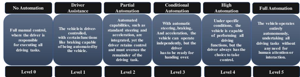
Figure 4. SAE automation levels for AVs.
