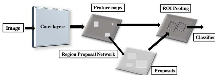
Figure 11. The architecture of Faster R-CNN [90].
