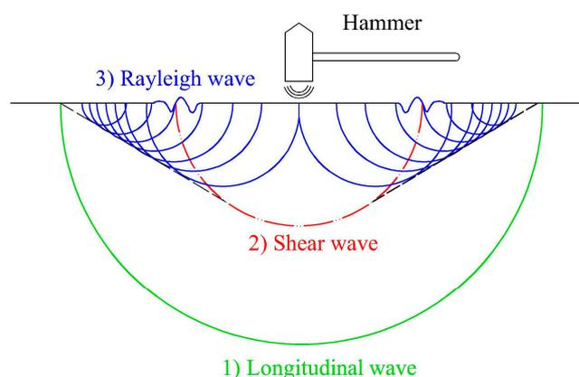
**Figure 15.** Types of stress waves in semi-infinite elastic material (based on [96]).
