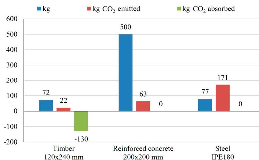
**Figure 1.** Weight, CO<sub>2</sub> emitted and absorbed by a 5 m span beam and 3 kN/m load [2]. Redrawn by the Timber Construction Research Group-UPM.
