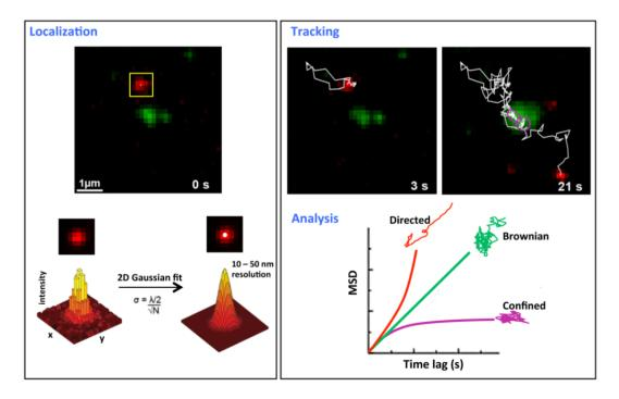
The advantage of SMT as compared to FRAP and FCS is that individual molecules can be analyzed with high spatial and temporal resolution providing a detailed description of their motion within the plasma membrane (Figure 1). SMT is based on the detection of individual molecules tagged with fluorescent markers using sensitive camera such as electron multiplied charge couple device (EMCCD) [21]. Typically, experiments are performed in low-density labeling conditions, resulting in a
