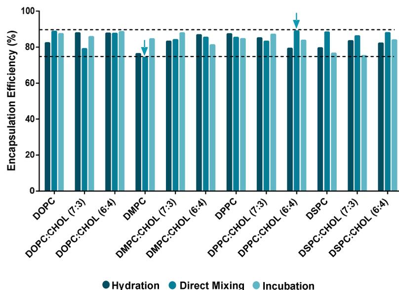
**Figure S2.** Encapsulation efficiency (EE %) of TDF (40  $\mu$ M) in liposomes with different degrees of membrane rigidity (4 mM) by three encapsulation methods: hydration, direct mixing and incubation. The dashed lines define the interval between the highest and lowest encapsulation efficiencies obtained.
