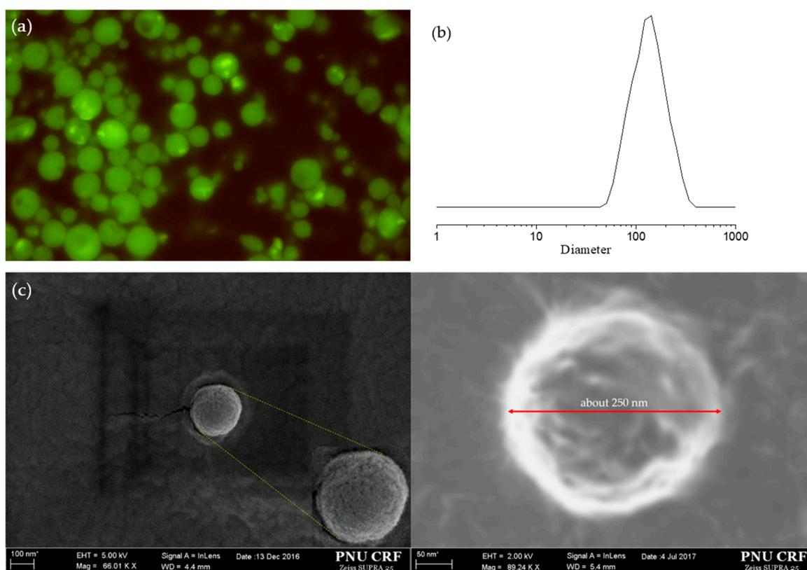
**Figure 5.** (a) Fluorescence microscopy, (b) DLS analysis, and (c) SEM images of FITC-BSA PFU nanoparticles.
