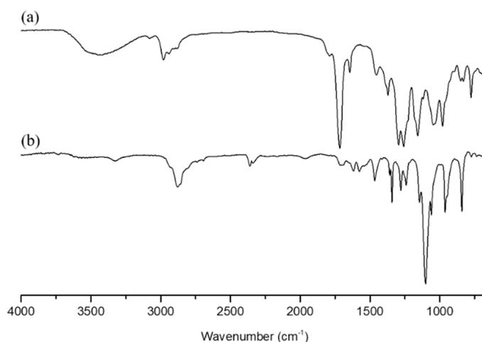
**Figure 1.** Fourier transform-infrared (FT-IR) spectra of (a) di-(2-hydroxypropyl fumarate) (DHPF) and (b) PFU.
