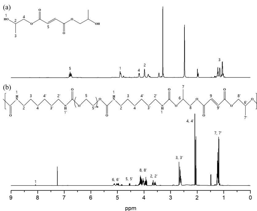
**Figure 2.**  $^1\text{H-NMR}$  spectra of (a) DHPF and (b) PFU.
