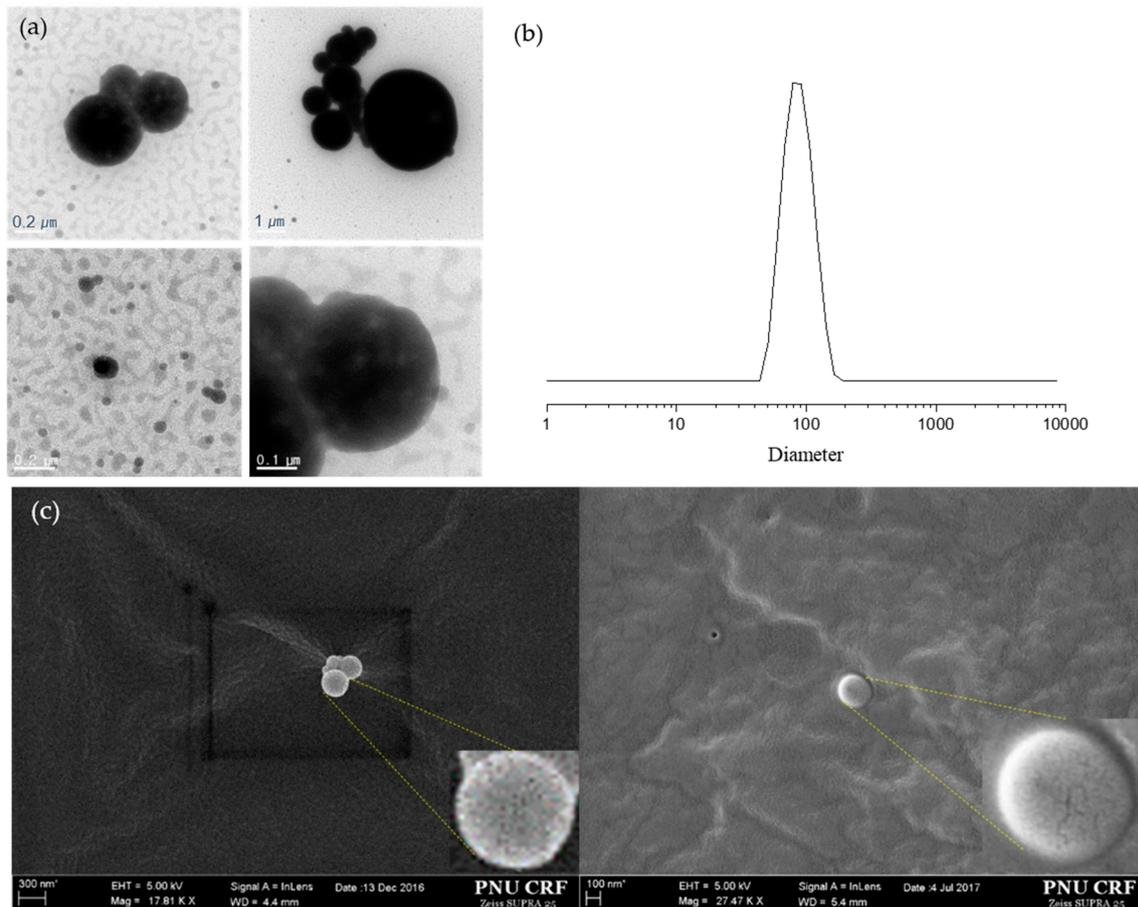
**Figure 4.** (a) TEM images, (b) DLS analysis, and (c) FE-SEM images of PFU nanoparticles.
