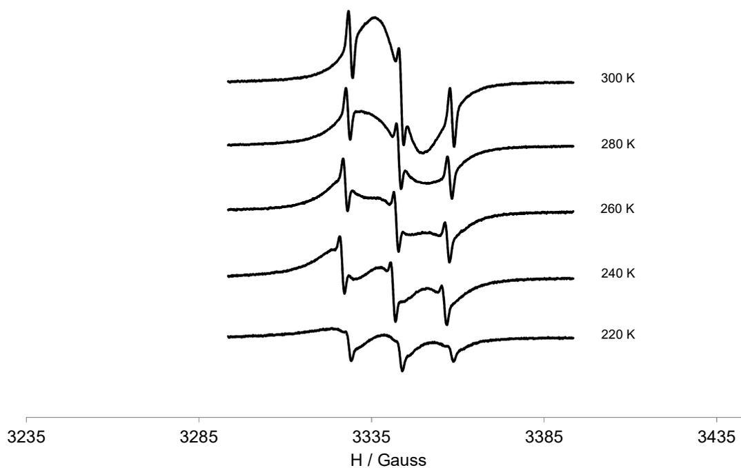
**Figure S8.** Variable temperature EPR spectra of G1-OEG-PROXYL from 300 to 220 K in  $\text{CH}_2\text{Cl}_2$ .
