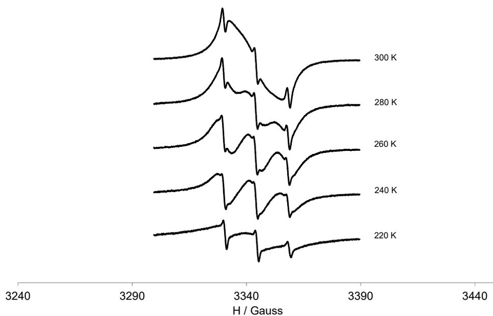
**Figure S7.** Variable temperature EPR spectra of G0-OEG-PROXYL from 300 to 220 K in  $\text{CH}_2\text{Cl}_2$ .
