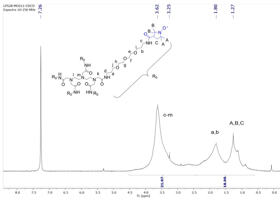
**Figure S6.**  $^1\text{H}$  NMR spectrum of G0-OEG-PROXYL-H dendrimer with their corresponding peaks assignment and relative integral values. The relative integral value for the group of protons (A,B,C + a,b) was found to be 18 and for the group of protons (c-m) 21.1, the same than the theoretical one 18: 22.
