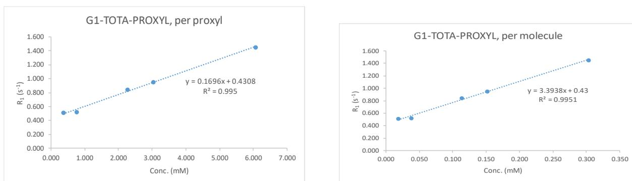
**Figure S11.** Plots of  $R_1$  of water molecules versus the nitroxyl radical unit (PROXYL) concentration (left) and the G1-OEG-PROXYL molecular concentration (right).
