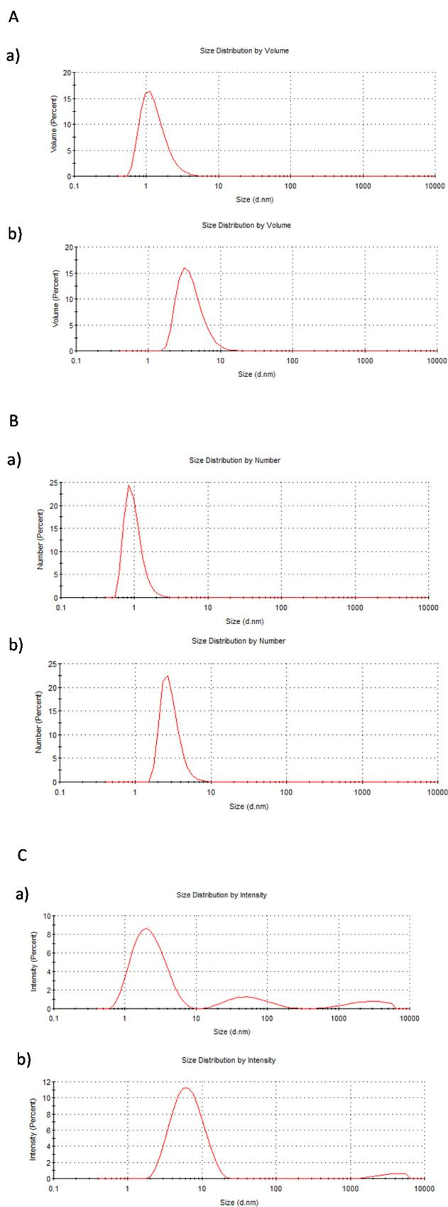
**Figure S3.** Mean diameters of G0-OEG-PROXYL (a) and G1-OEG-PROXYL (b) determined by DLS, from the size distribution by volume (A), by number (B) and by intensity (C) at 25 °C in PBS.
