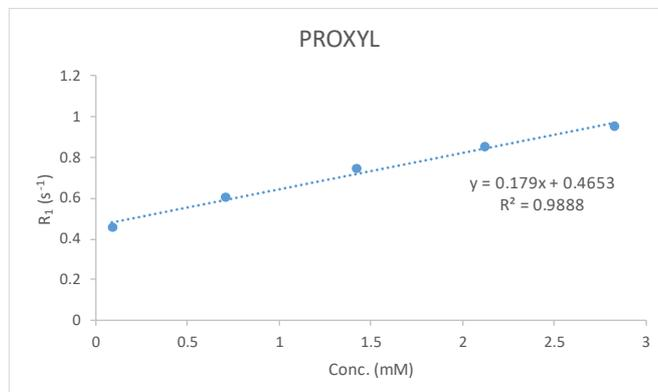
Figure S9. Plots of R<sub>1</sub> of water molecules versus PROXYL concentration.
