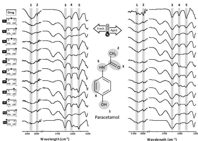
**Figure 1.** FTIR of the paracetamol as supplied and the effervescent extrudates obtained according to a combined mixture design before and after aging.
