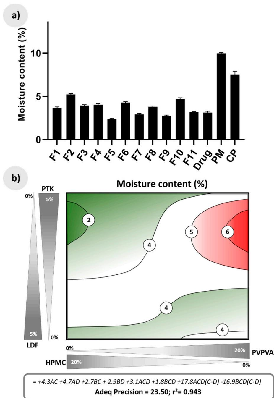
**Figure 4.** (a) Moisture content (%) of the drug as supplied, the physical mixture containing drug and effervescent salts (PM), commercial drug product (CP), and effervescent extrudates after aging; (b) Response surface for moisture content according to a linear-cubic model, together with its predictive equation (A = PVPVA, B = HPMC, C = PTK, and D = LDF). The green regions show compositions with low moisture levels, and the red regions indicate compositions with high moisture levels.
