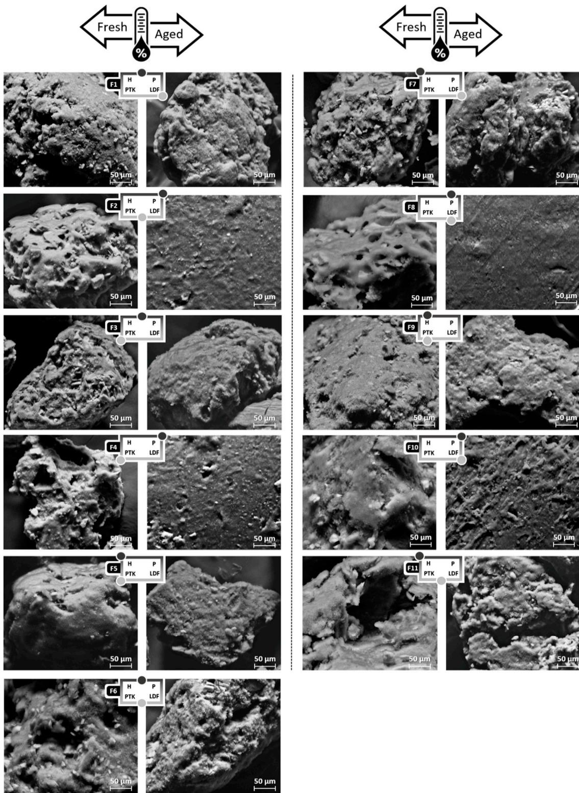
**Figure 3.** SEM photomicrographs of effervescent extrudates obtained according to a combined mixture design before and after aging at a 1000× magnification.
