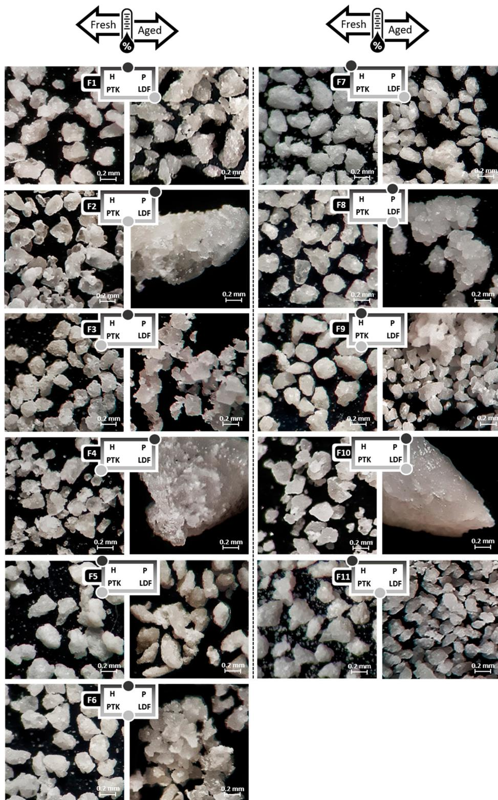
Figure 2. Optical microscopy photomicrographs of effervescent extrudates obtained according to a combined mixture design before and after aging at a 45× magnification.
