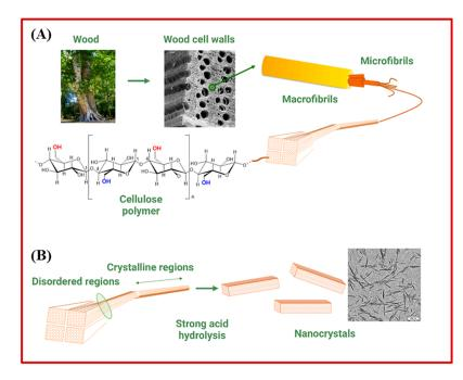
**Figure 2.** (**A**) The hierarchical structure of cellulose nanofibers derived from the tree. (**B**) The fabrication of cellulose nanocrystals (CNCs) from the nanofibrous network using acid. Adapted with permission from Ref. [57], Copyright 2015, Intech.
