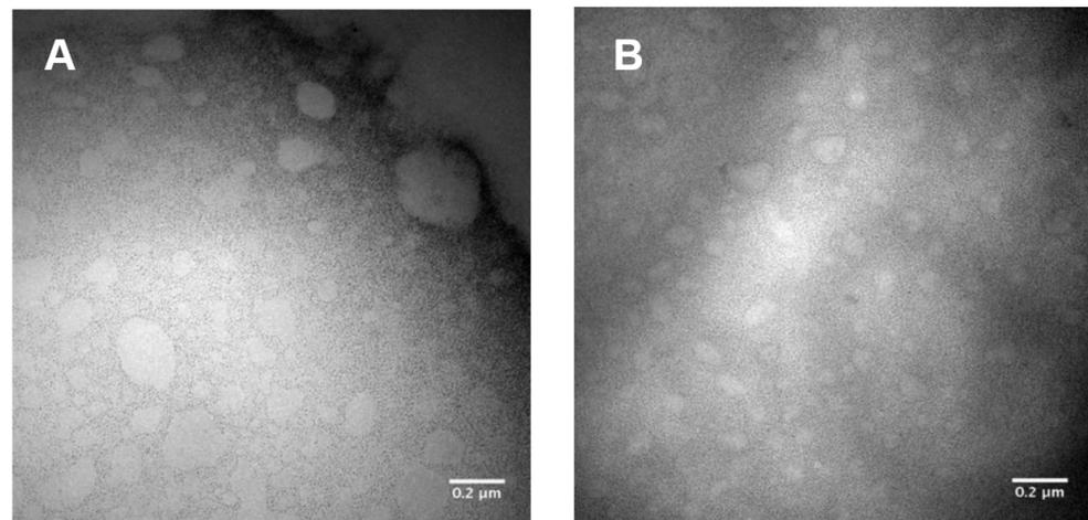
**Figure 1.** Representative images obtained by transmission electron microscopy of samples diluted 100 times in distilled water. Nano-1 (A) and Nano-2 (B). One hundred thousand times increase.
