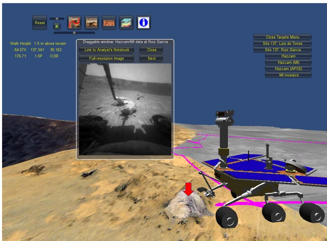
A fourth function of the Santa Maria VA is the ability to measure the distance between two points. This allows the user to measure the size of objects like rocks in the scene. To use this function the user first left click on a point in the scene and then drag the mouse to a second point. Both points are marked in red on the screen for reference. The system will then calculate the distance between two points and display the result on the screen in a pop-up window as shown in Figure 11.
