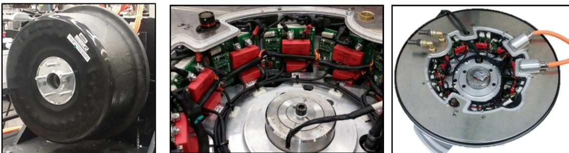
Figure 2. Back and front Evolution 1 (EVO 1) plus integrated power electronics.
