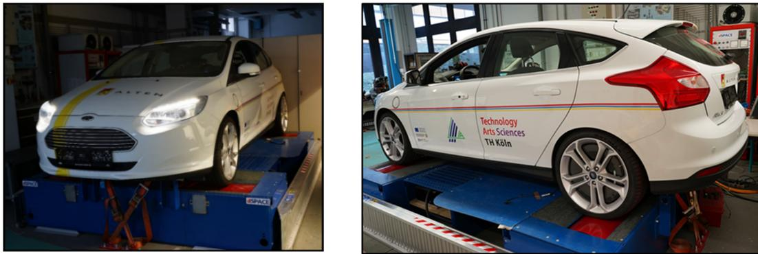
Figure 7. Project demonstrator on roller test bench.
