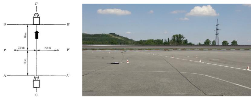
**Figure 12.** Measurement layout [9] (Reproduced from Official Journal of the European Union; published by EU-Norm, 2014) and practical test at the Aldenhoven Proving Ground.
