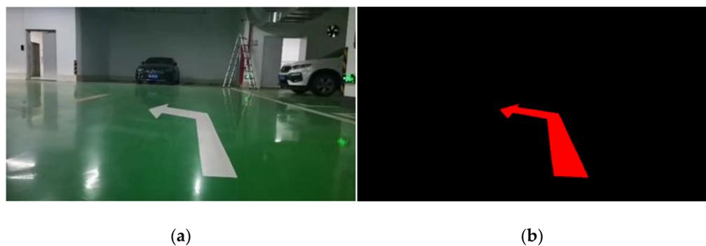
**Figure 14.** Before and after lane line detection. (a) Image to be detected. (b) Renderings of lane line detection.
