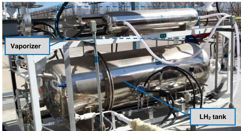
Figure 2. Equipment of original LH<sub>2</sub> system.
