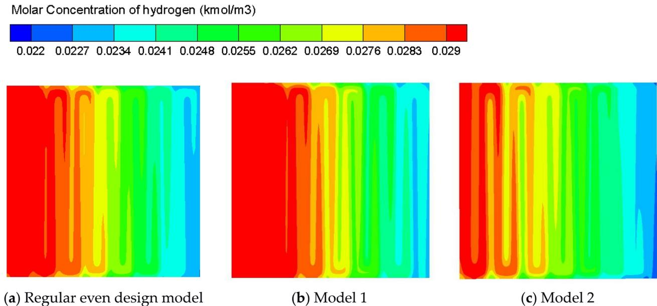
**Figure 4.** H<sub>2</sub> concentration distribution on the anode gas diffusion layer.
