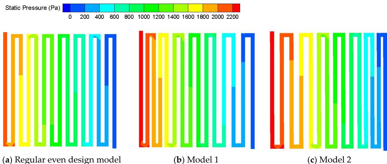
Figure 3. Pressure distribution in the cathode flow channel.
