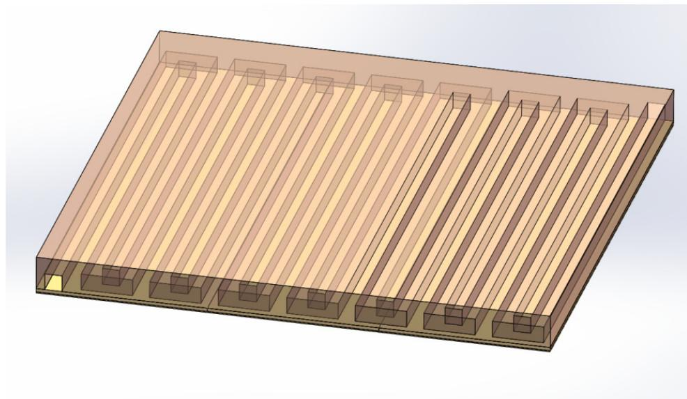
**Figure 1.** Schematic diagram of the PEMFC anode structure.
