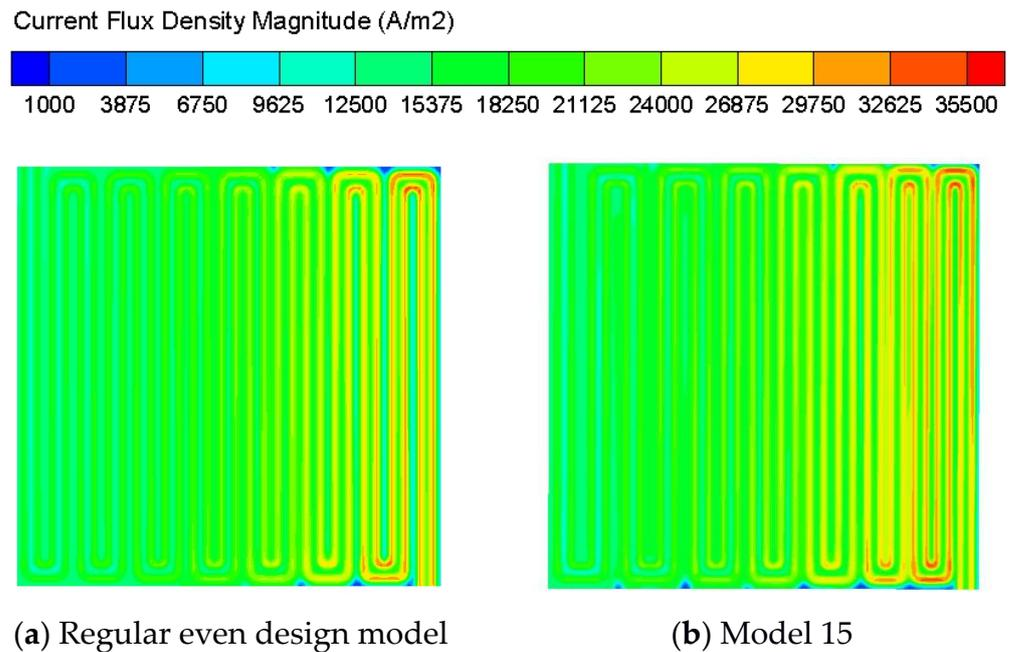
**Figure 5.** Current density distribution on the cathode catalyst layer.
