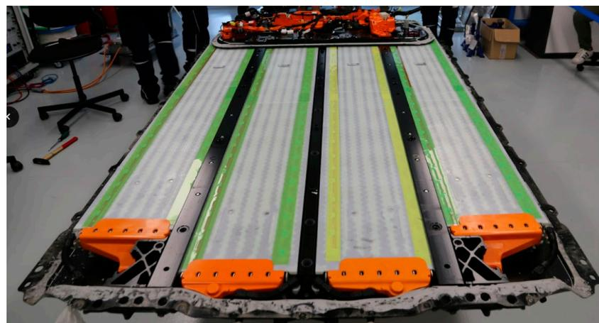
**Figure 9.** Tesla Model 3 unassembled battery pack.
