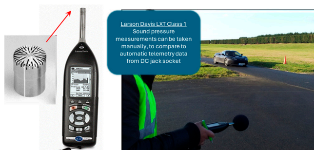
Figure 5. Sound pressure meter and setup on location.
