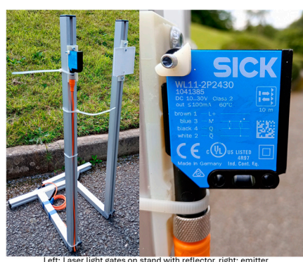
Figure 6. Laser light proximity gates used to measure when the vehicle enters and leaves the test area (digital signal as open/closed).
