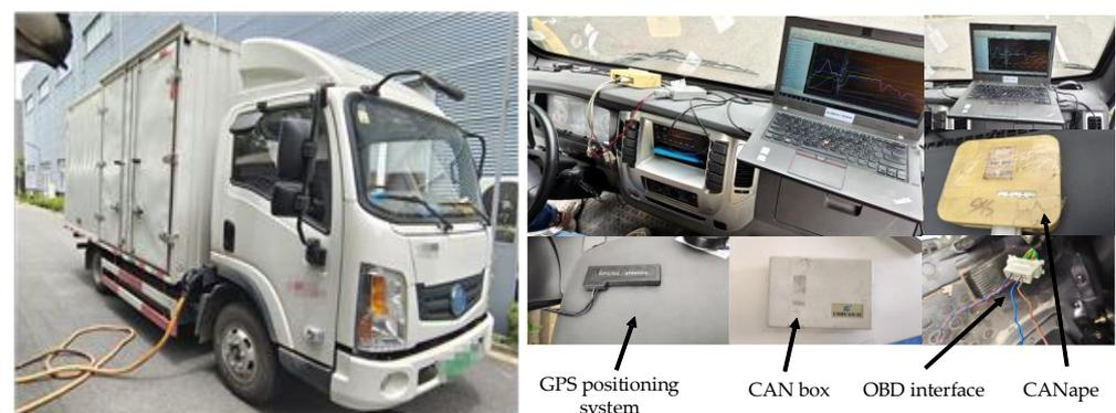
**Figure 9.** Test vehicle and real vehicle test platform.
