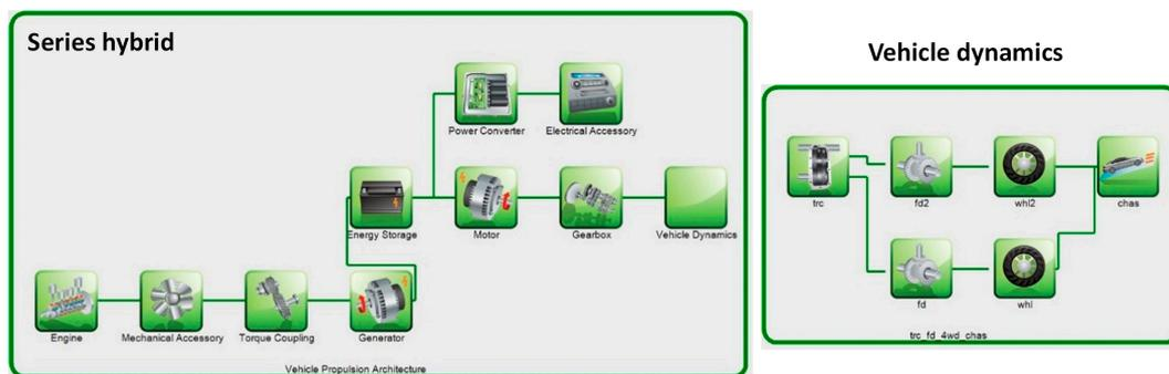
**Figure 2.** Series hybrid powertrain layouts and vehicle dynamics block layouts of the tractor models.
