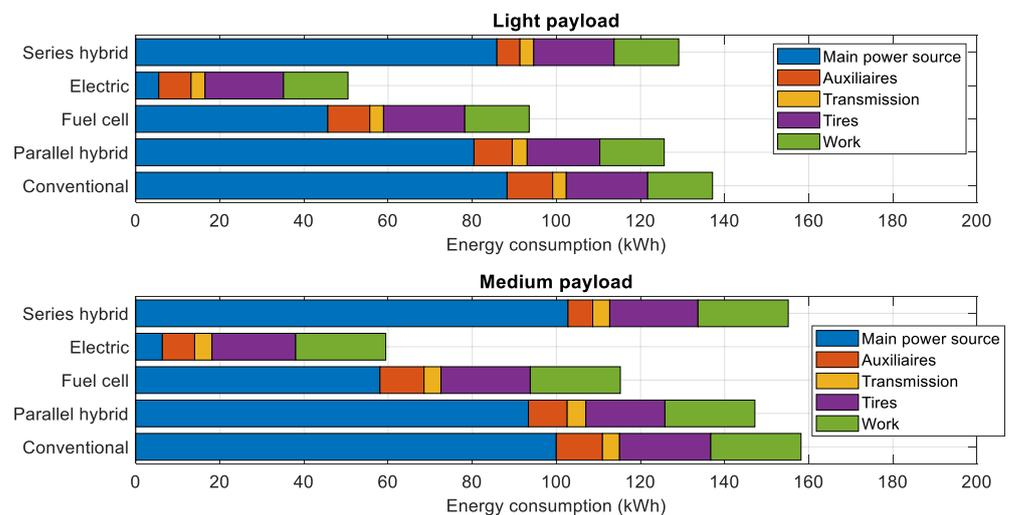
**Figure 14.** Distribution of energy losses for the different large tractor models in the Road cycle with two payloads.
