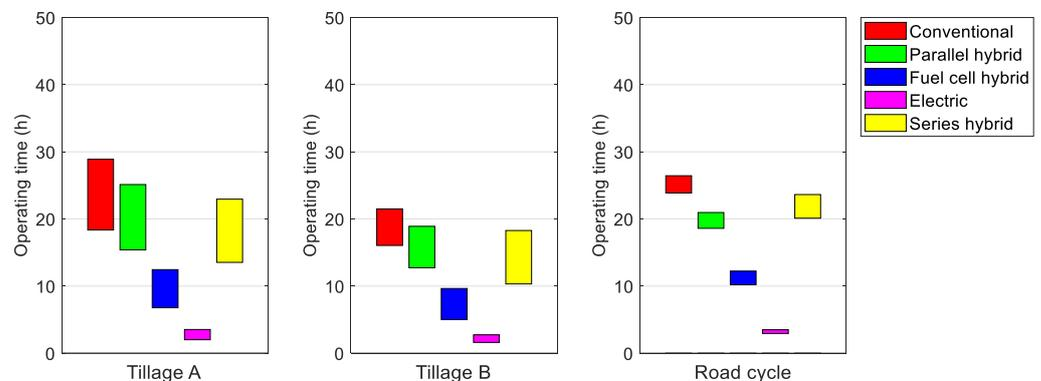
**Figure 16.** Calculated variations in operating times for different cycles for the medium-sized tractor.
