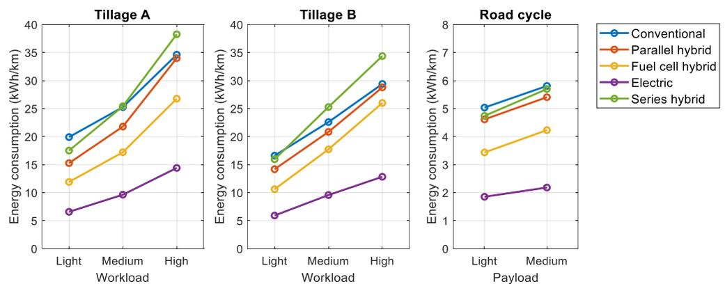
**Figure 9.** Energy consumption in kWh/km for all simulated cycles for the large-sized tractor.
