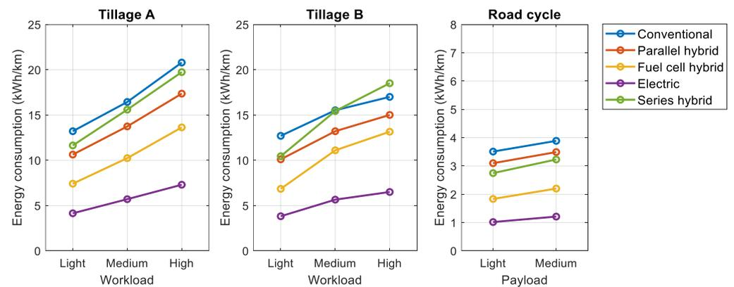
**Figure 10.** Energy consumption in kWh/km for all simulated cycles for the medium-sized tractor.
