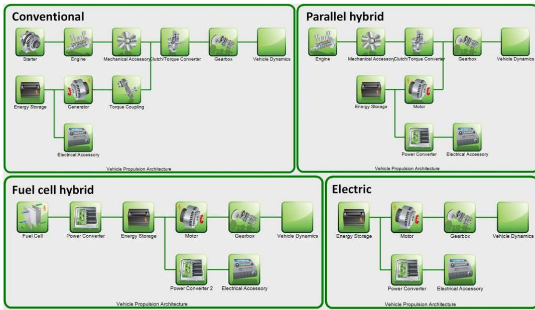
**Figure 1.** Powertrain layouts of the conventional, parallel hybrid, fuel cell hybrid, and electric tractor models in the Autonomie software.
