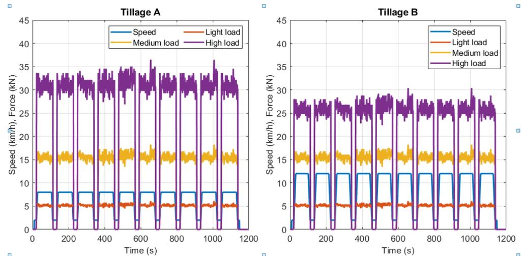
**Figure 4.** Generated tillage cycles (Tillage A and B) with three defined load resistance profiles for the large-sized tractor.
