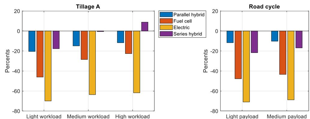
**Figure 12.** Potential for reducing energy consumption in the Tillage A and Road cycles of the medium-sized tractor.
