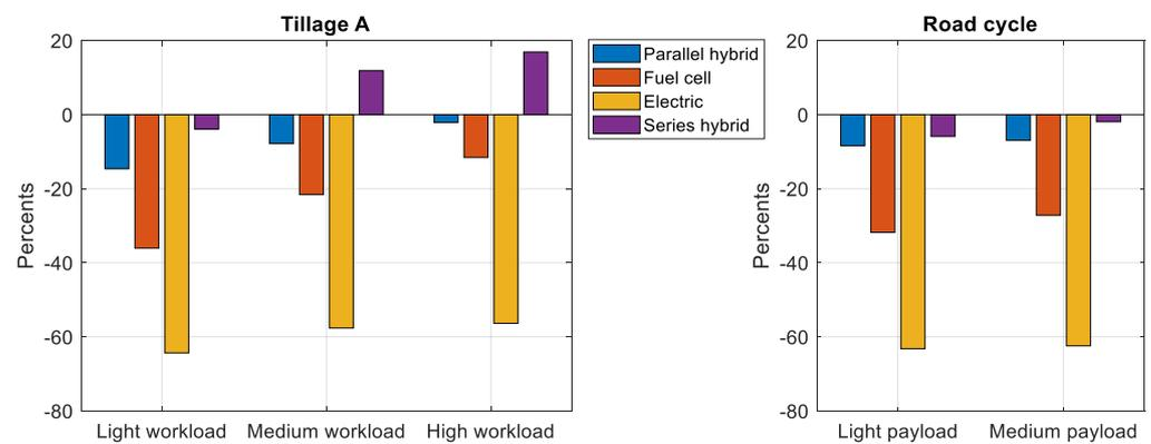
**Figure 11.** Potential for reducing energy consumption in the Tillage A and Road cycles of the large-sized tractor.
