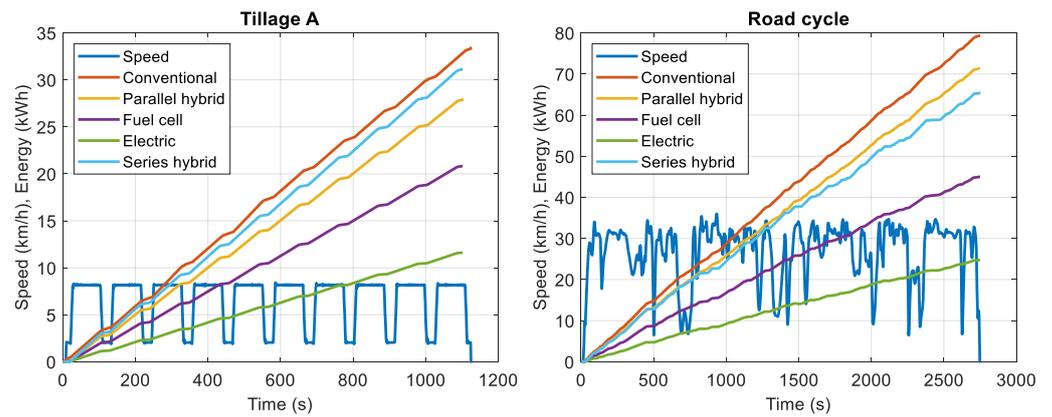
**Figure 8.** Cumulative energy consumption in the Tillage A and Road cycles for the medium-sized tractor models.
