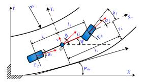
Figure 1. Two-degrees-of-freedom model of vehicle.
