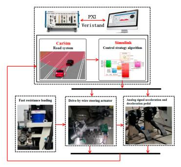
Figure 12. Schematic diagram of the test architecture.
