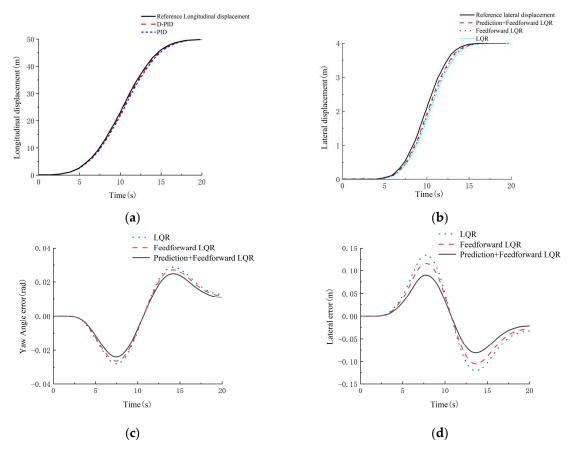
**Figure 8.** Trajectory tracking curve for condition 1. (a) Comparison of longitudinal displacement; (b) comparison of lateral displacement; (c) transverse pendulum angle error; (d) lateral error.
