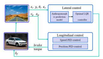
Figure 6. Trajectory tracking controller.
