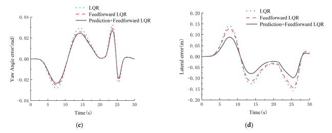
**Figure 10.** Trajectory tracking curve for condition 2. (a) Comparison of horizontal line displacements; (b) longitudinal velocity comparison diagram; (c) transverse pendulum angle error; (d) lateral error.
