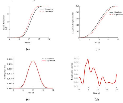
**Figure 13.** A graph of the bench test results. If there are multiple panels, they should be listed as (a) comparison of lateral displacement; (b) comparison of longitudinal displacement; (c) transverse swing angle comparison chart; (d) vertical error.
