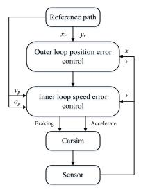
Figure 5. Vertical tracking control framework.
