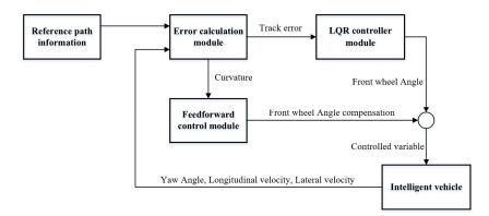
Figure 2. Lateral tracking control algorithm flow.
