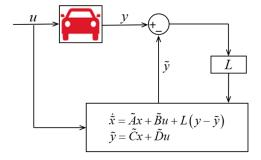
Figure 4. Schematic diagram of the Luenberger observer.
