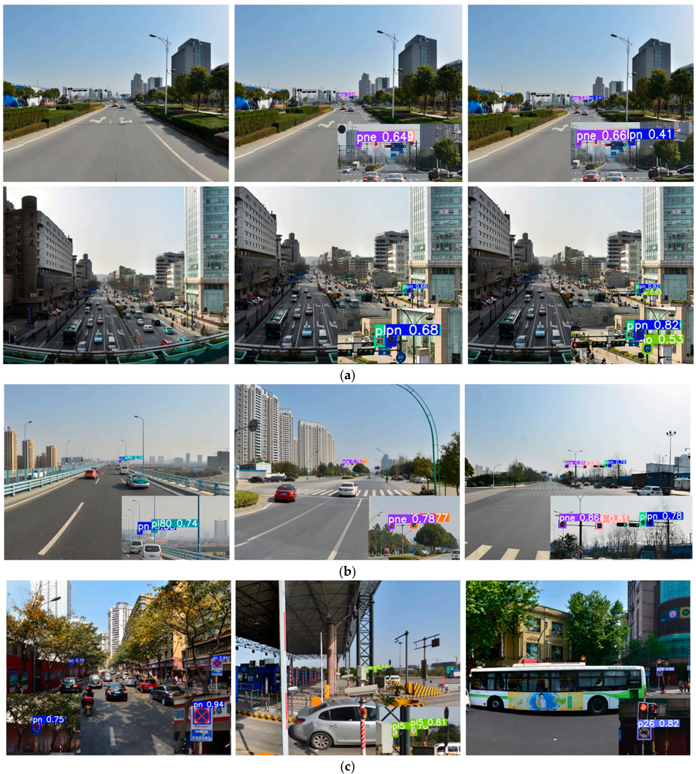
Figure 10. Visualization outcomes on the TT100K dataset include (a) a comparative analysis of the results between YOLOv5s and YOLO-ADual, (b) detection outcomes for small targets, and (c) detection performance in challenging conditions such as shadows, occlusions, and cloudy weather.
