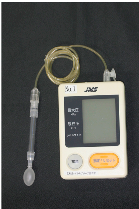
Figure 1. Devices and methods for measuring the lip seal strength and tongue pressure. (a) Measurement of lip seal strength. (b) Measurement of tongue pressure (the device displays current and maximum pressures).
