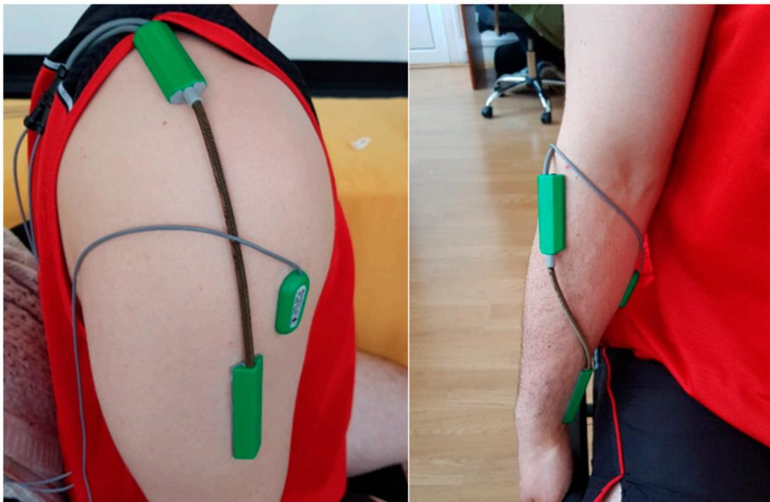
**Figure 20.** Sensors positioning on the upper limb (on the left the two axis goniometer for the shoulder motions and on the right the torsionmeter for the forearm motion).
