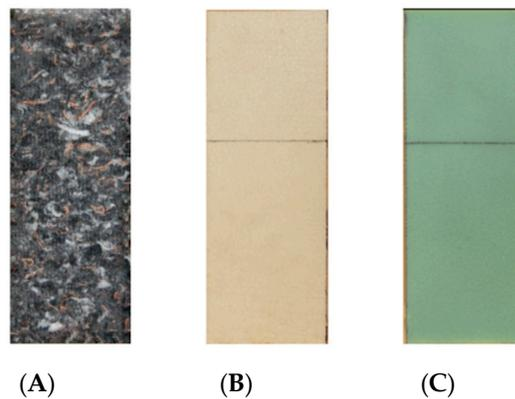
**Figure 2.** Test samples (A)—Senizol AT XX2 TL 60, (B)—polystyrene, (C)—polyurethane foam.
