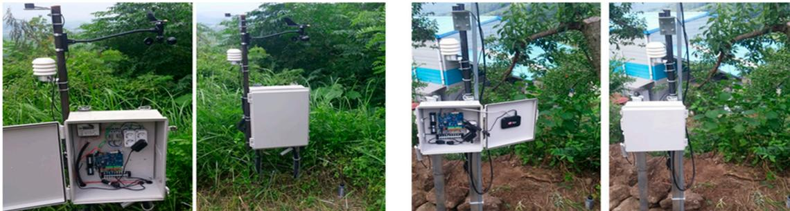
**Figure 8.** Units of IoT-based, specialized-fruit-integrated management platform.
