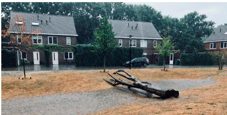
**Figure 6.** Example of temporary rainwater conservation and infiltration in “wadi’s” on slopes in Ede, The Netherlands (picture Koen Claassen).
