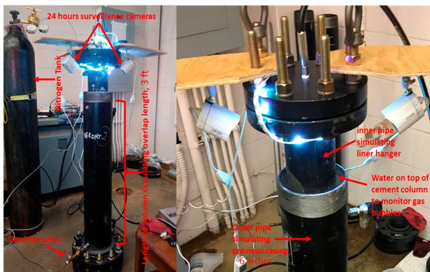
**Figure 3.** Experimental setup used to simulate the liner hanger–casing overlap.
