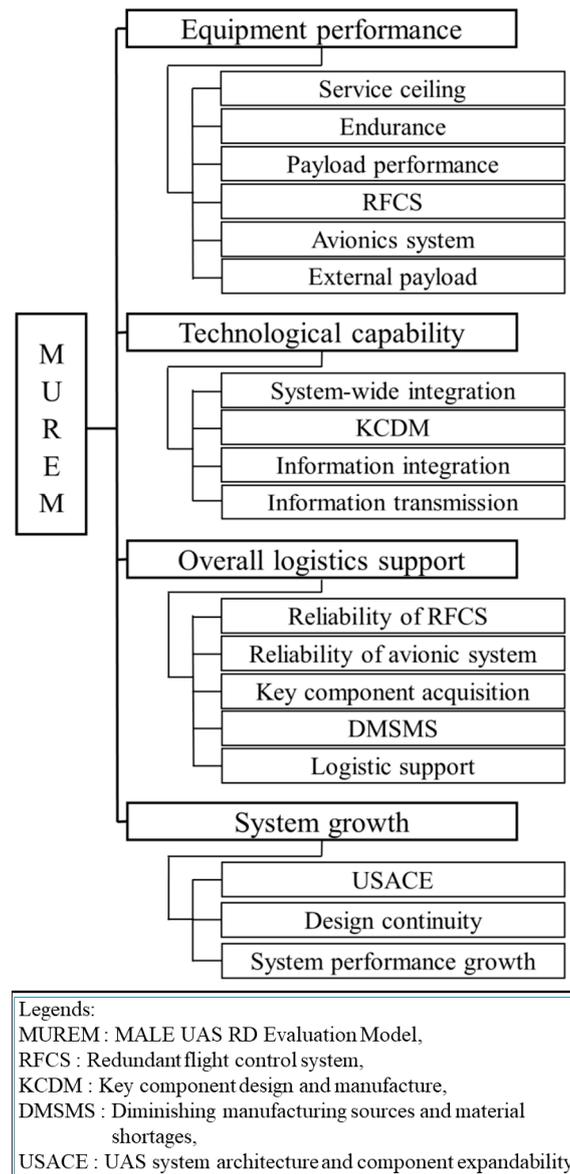
**Figure 5.** The decision hierarchy for medium-altitude long-endurance unmanned aerial system (MALE UAS) design.
