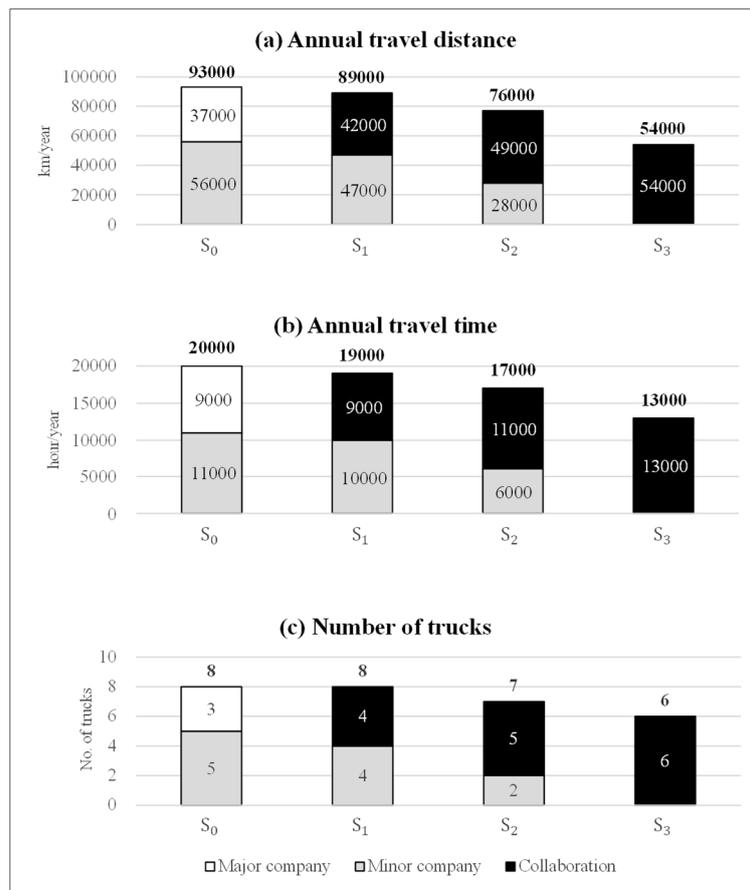
Figure 5. (a) annual travel distance; (b) annual travel time; (c) number of trucks for delivery under various levels of collaboration.
