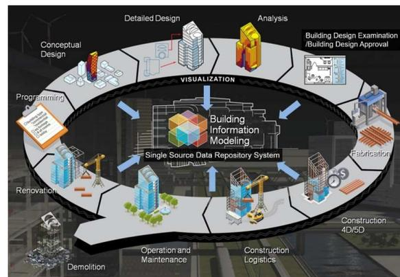
**Figure 1.** Building Information Modelling (BIM) life cycle workflow diagram (modified from Autodesk).
