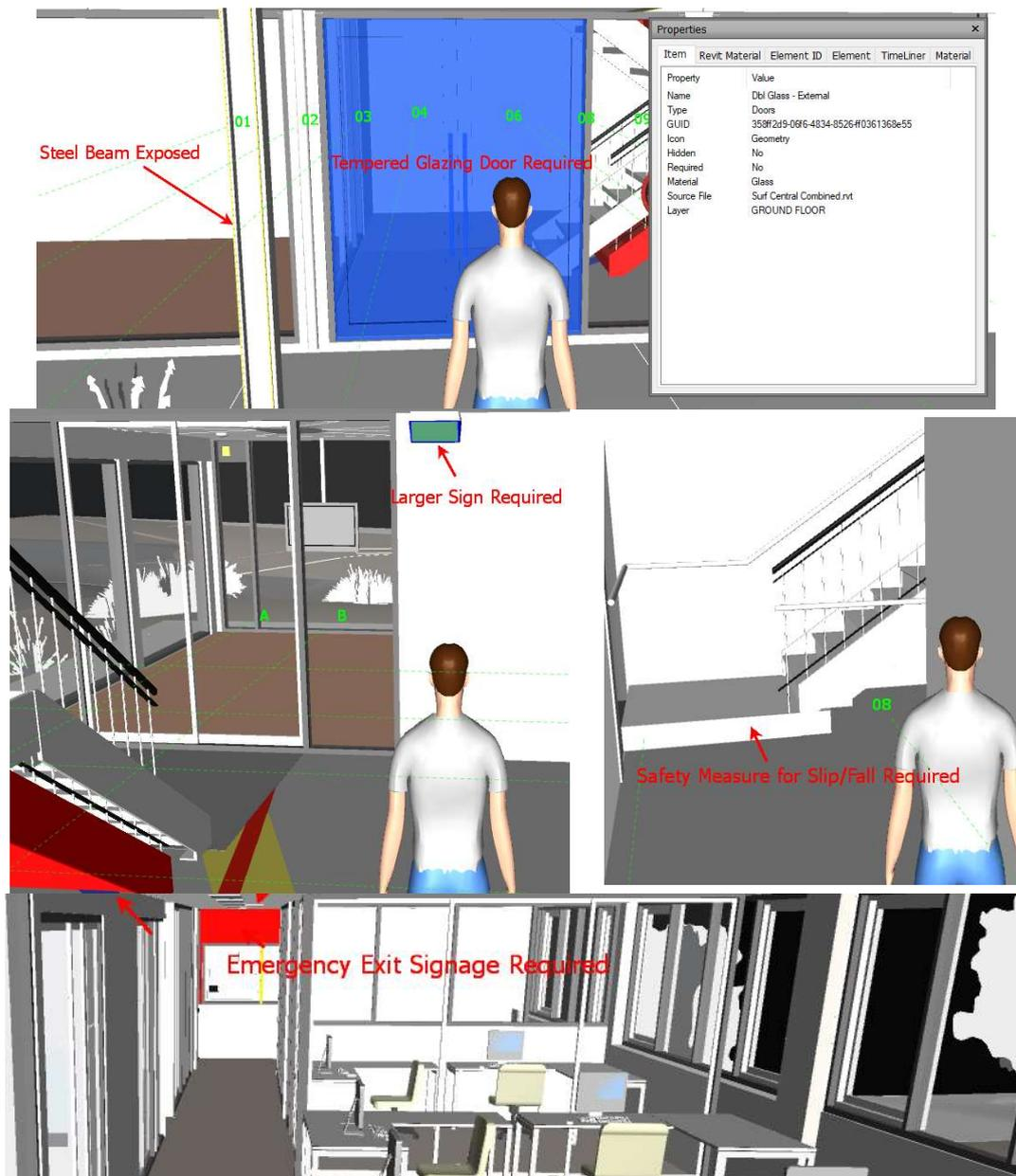
**Figure 8.** BIM-enabled co-investigation results (top: Entrance of building; middle left: Emergency exit sign; middle right: Stair and step; bottom: Emergency exit signage on the second floor).
