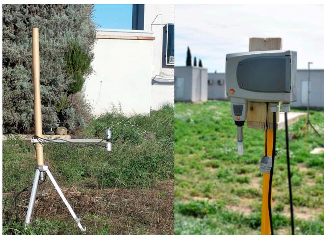
**Figure 6.** On the left, Middleton Solar meter. On the right, Testo 6651 for air temperature and relative humidity.
