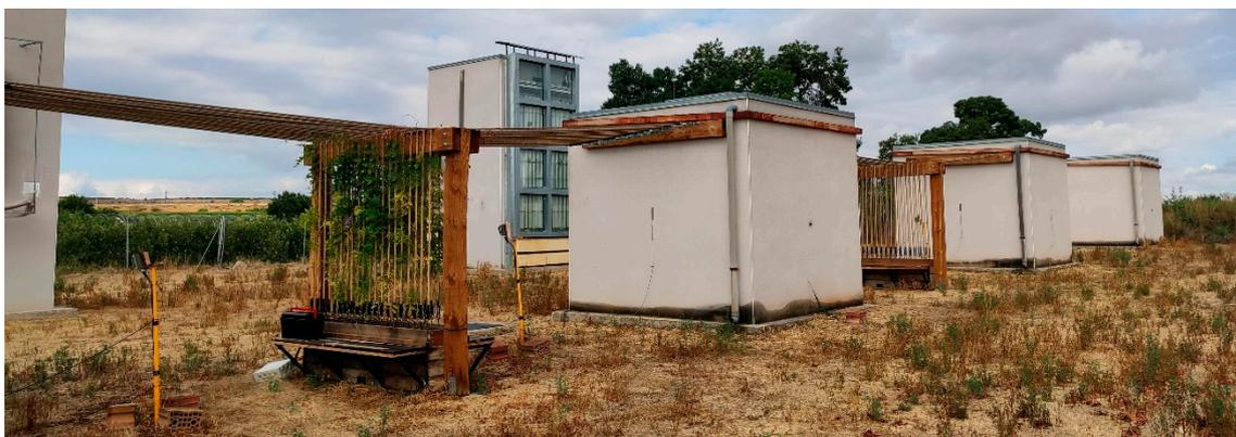
**Figure 2.** The two shadow systems, on the left with greenery and on the right without greenery.
