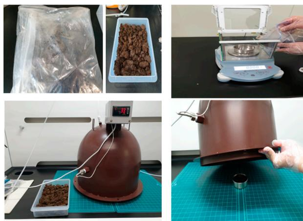
Figure 8. Ammonia flux estimation experiment using a field sample.
