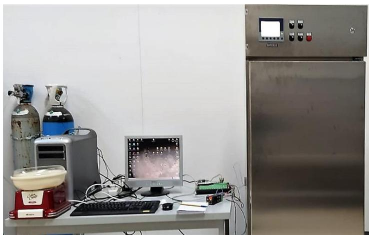
**Figure 1.** Image of the completely assembled experimental apparatus (from left to right: A device for making cotton candy, a PC, a data logger, a Hall effect sensor, a PID controller, and a climatic chamber).
